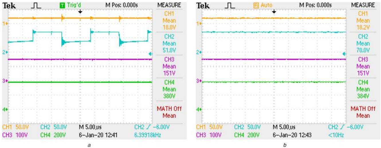
**Fig. 6** Experimental waveforms obtained from the prototype converter to validate the voltage gain at various locations
