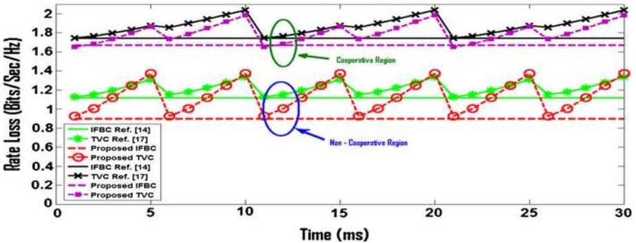
Fig. 4 Rate loss versus sub-frame index  $T_s$  when  $B_{res} = B_{res,TVC} = 8$ ,  $\tau_{l,i,i} = 5$ ,  $\tau_{l,i,j} = 10$ ,  $\eta_{l,i,i} = \eta_{l,i,j} = 0.99$  and  $\gamma_{l,i,i}, \gamma_{l,i,j}(r_i, r_j = 500) = 10$  dB
