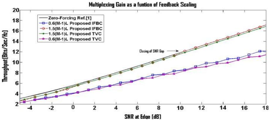
Fig. 8 Feedback scaling for multiplexing gain when  $\tau_{l,i} = \tau_{l,j} = 2$ ,  $\eta_{l,i} = \eta_{l,j} = 0.99$
