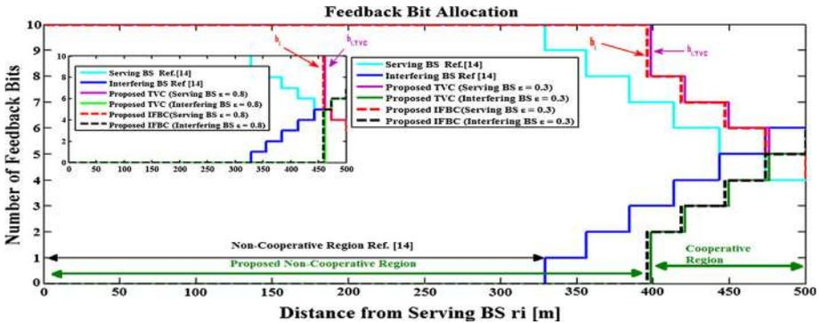
**Fig. 2** Feedback allocation strategy for IFBC for various  $\epsilon$  when  $\gamma_{l,i,j}(r_i = 500) = 10$  dB and  $\gamma_{l,i,j}(r_j = 500) = 10$  dB,  $\tau_{l,i,i} = \tau_{l,i,j} = 10$
