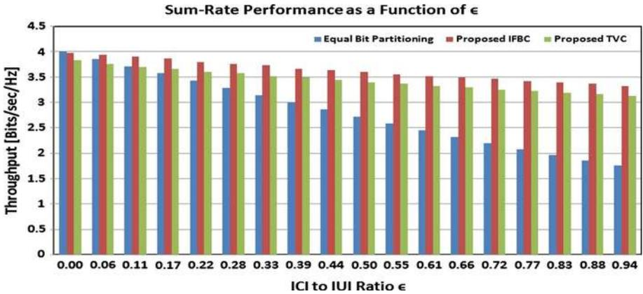
Fig. 3 Sum-rate against  $\epsilon$  for  $B_{res} = B_{res,TVC} = 8$ ,  $\tau_{l,i,i} = \tau_{l,i,j} = 2$ ,  $\gamma_{l,i,i}(r_i = 500) = 10$  dB and  $\gamma_{l,i,j}(r_j = 500) = 10$  dB
