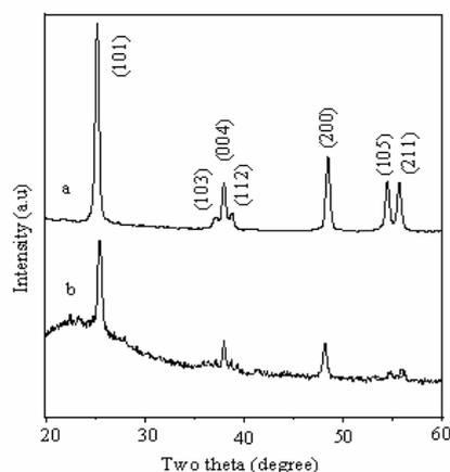
Fig. 1 XRD pattern of  $\text{TiO}_2$  and  $\text{TiO}_2@SiO_2$
