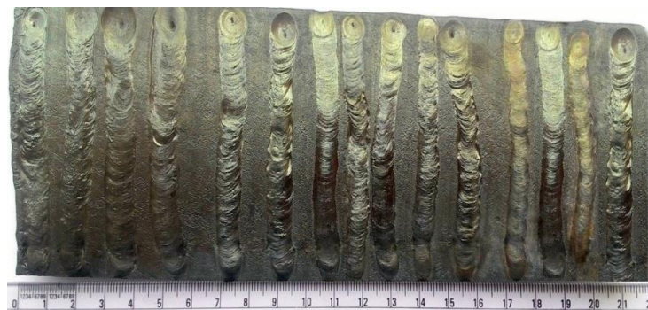
Figure 1. Photograph showing the bead-on-plate trial welds over C300.
