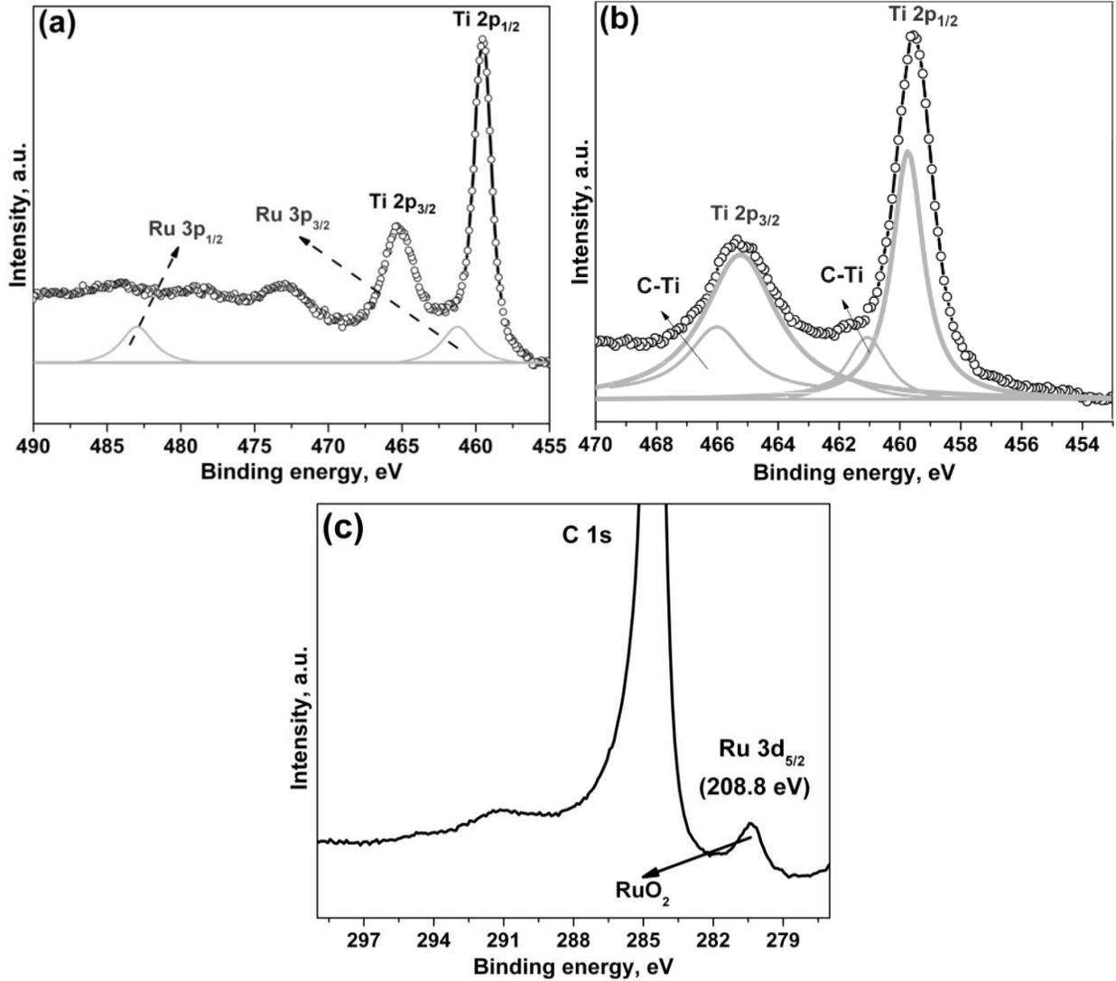
**Fig. 4** XPS spectrum of  $\text{TiO}_2/\text{u-RuO}_2/\text{GNS}$ ; main peaks of (a) Ru 3p and Ti 2p, (b) Ti 2p, and (c) C 1s
