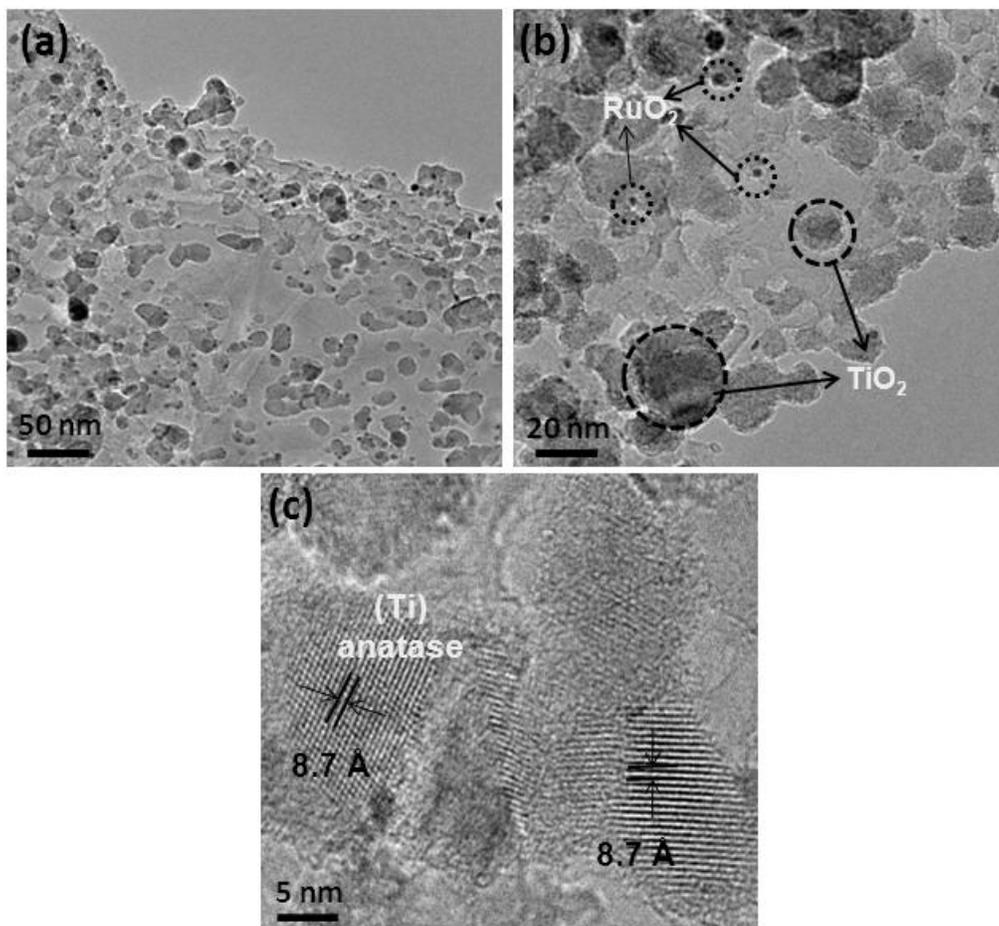
**Fig. 2** TEM images of  $\text{TiO}_2/\text{u-RuO}_2/\text{GNS}$
