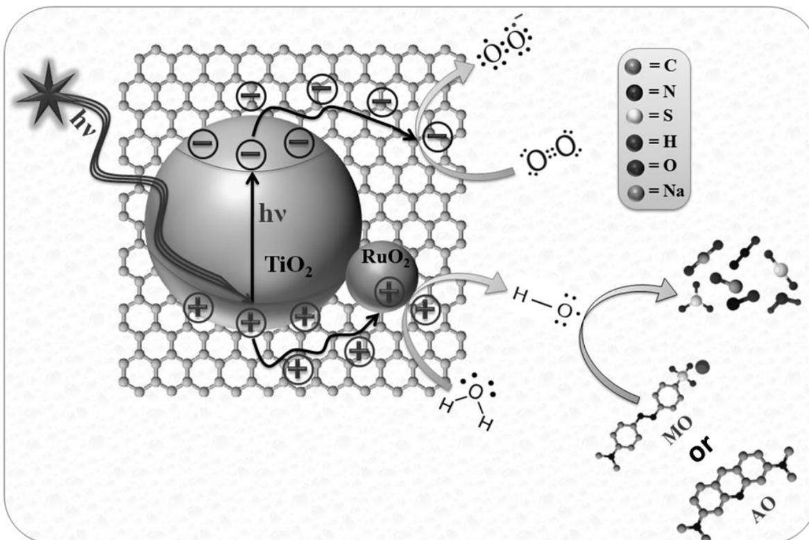
**Fig. 7** Photocatalytic degradation of organic pollutants using  $\text{TiO}_2/u\text{-RuO}_2/\text{GNS}$
