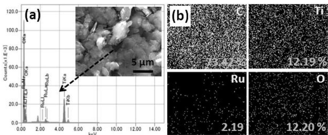
**Fig. 3** (a) SEM (inset) and EDS spectrum of  $\text{TiO}_2/\text{u-RuO}_2/\text{GNS}$  and (b) corresponding elemental mapping observations of C, Ti, Ru and O
