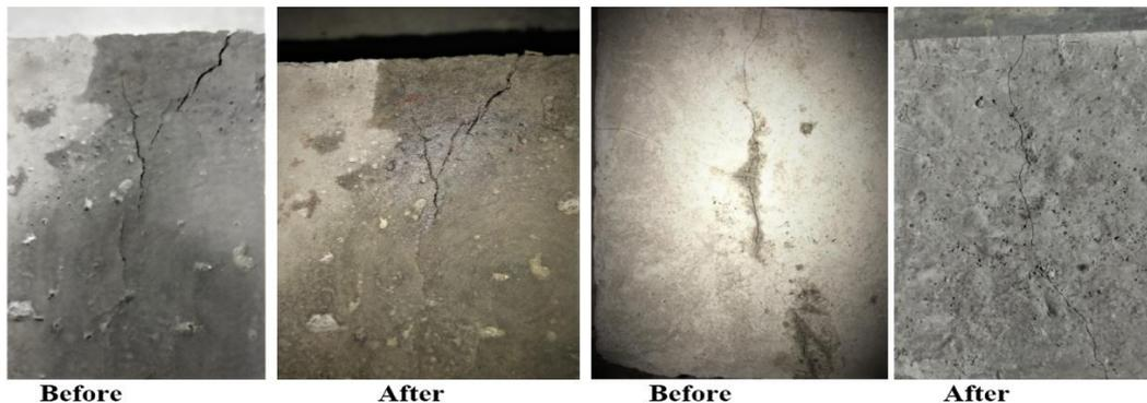
**Figure 12.** Cracks visibility before and after curing in a room atmosphere for 28 days.
