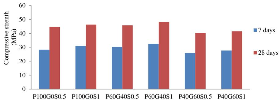
**Figure 7.** Graphical representation of compressive strength with various proportions of SAPs.
