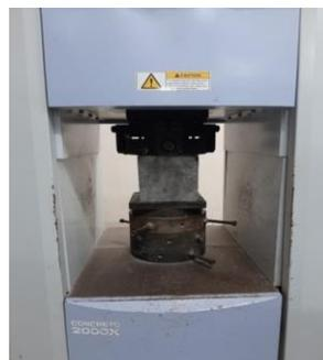
**Figure 5.** The test set up in CTM.
