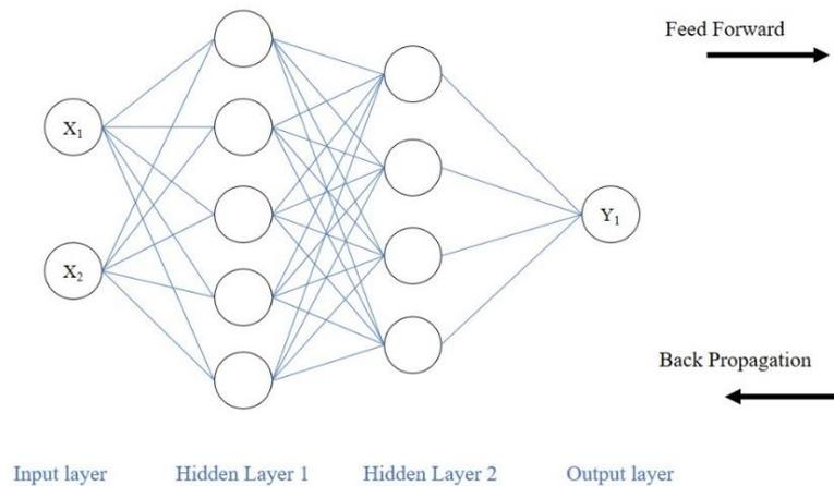
**Figure 3.** Selected ANN model for the prediction of Pozzolanic strength properties.
