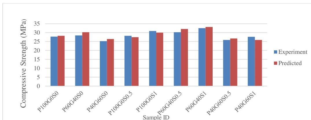
**Figure 13.** Comparison of Predicted and Experimental 7 day compressive strength.
