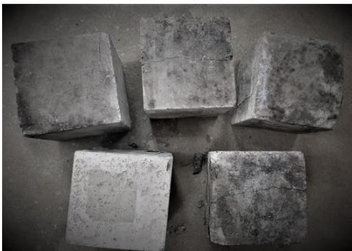
**Figure 9.** Cracked cubes in room temperature.
