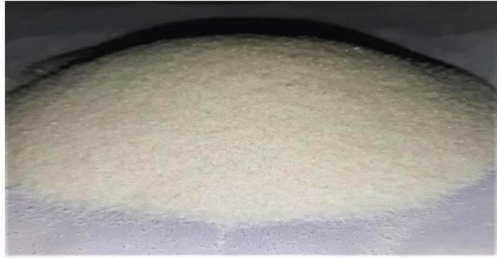
**Figure 2.** Super Absorbent Polymer.
