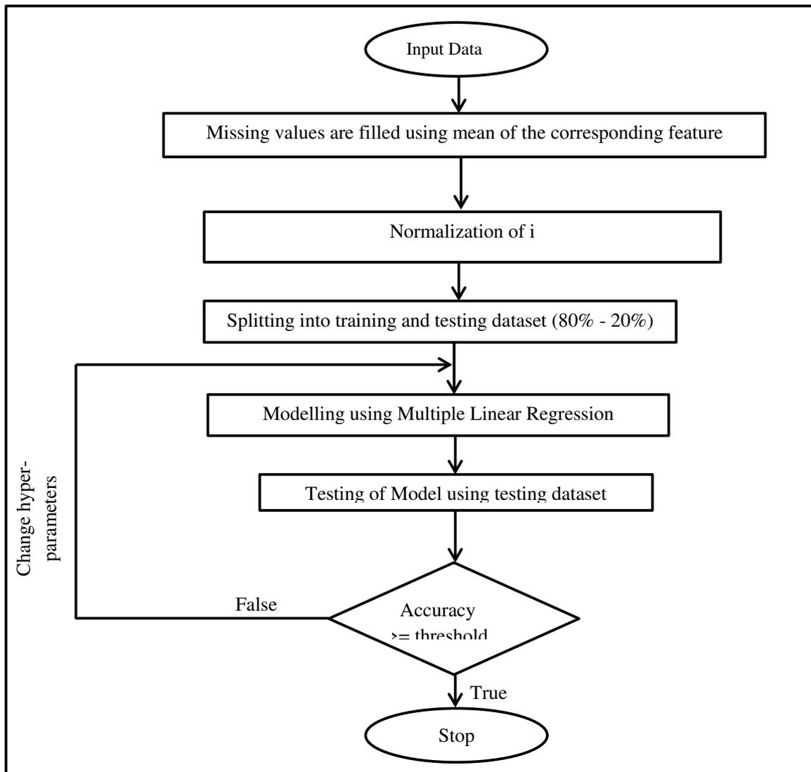
Figure 3. Process flow diagram of Predictive Model
