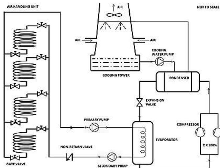
**Figure 1.** Schematic diagram of Chiller Plant
