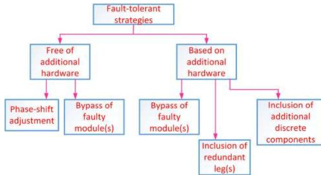
**Fig. 11** Categorisation of fault-tolerant strategies available in literature for DC–DC converters
