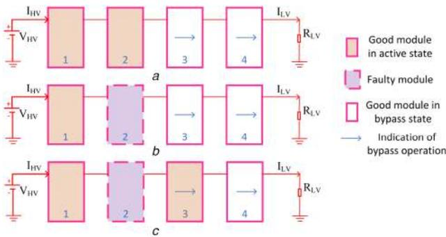
**Fig. 14** Fault bypass operation and redundancy of MMC [100]
