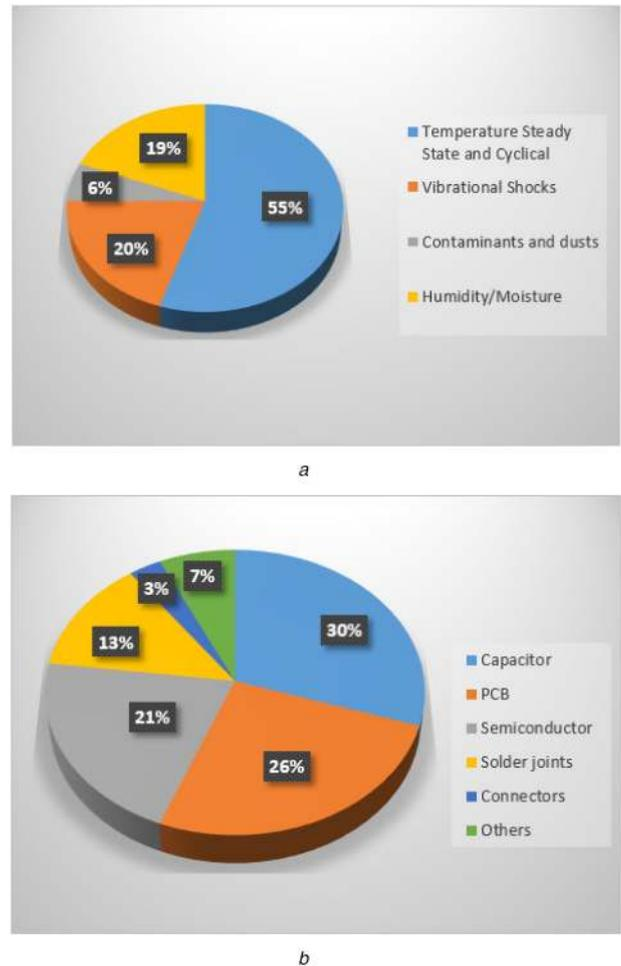
Fig. 1 Stress distributions and failure in power electronic systems [6, 7] (a) Source of stress distribution, (b) Failure root cause distribution
