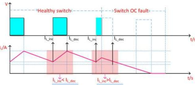
**Fig. 6** Inductor current evolution in non-isolated unidirectional buck converter, under healthy and faulty conditions
