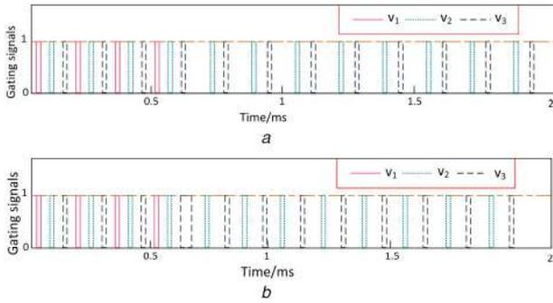
**Fig. 12** Interleaved switching pattern after OCF at  $t = 0.55$  ms
