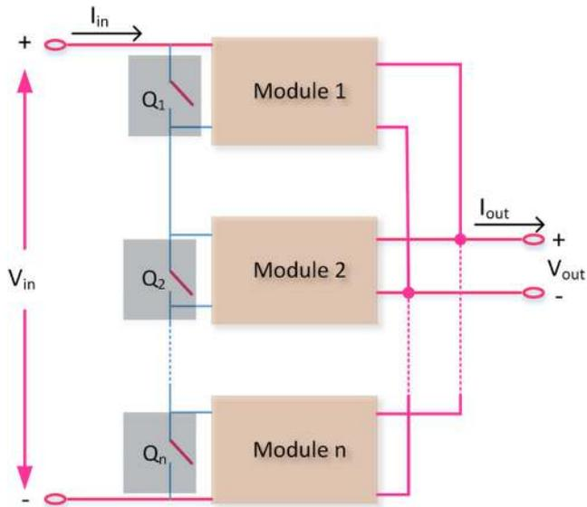
**Fig. 15** Fault-tolerant implementation in input series output parallel converter [102, 103] ( $Q_1, Q_2, Q_n$  denotes the bypass switches)
