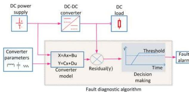
**Fig. 10** Development of model-based fault diagnostic algorithm for DC–DC converters
