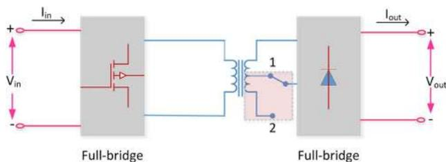
**Fig. 16** FTO of full bridge DC-DC converter depends on auxiliary winding connected in secondary winding of transformer [39]
