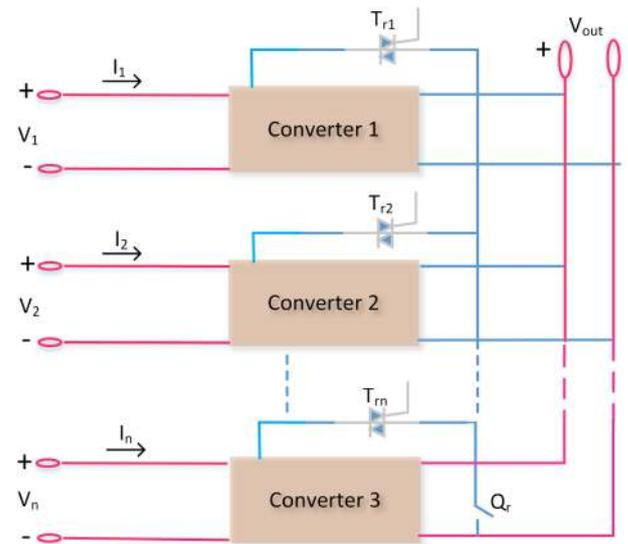
**Fig. 18** Redundant leg implementation depends on simple redundant switch [40]
