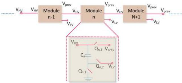
**Fig. 13** Bidirectional MMC Fault-tolerant structure [99]
