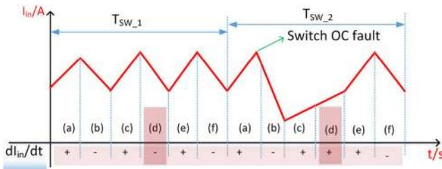
**Fig. 8** Development of input current in time for 3-phase interleaved boost converter in two switching intervals. Highlighted the OC fault by shadowed portions during the  $T_{SW\_2}$  period [51]
