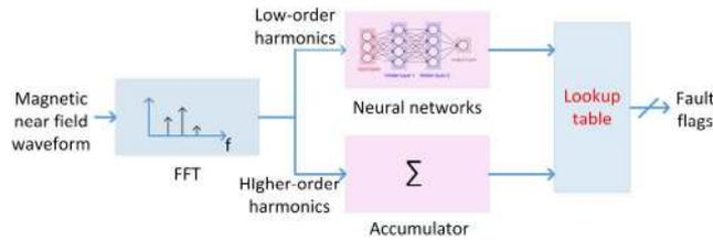
**Fig. 9** Spectral evaluation of MNF waveform fault diagnostic algorithm
