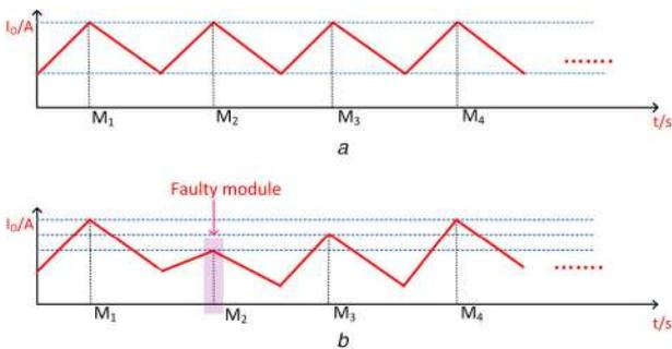
**Fig. 7** Parallel connected single active bridge output current under various conditions [51]
