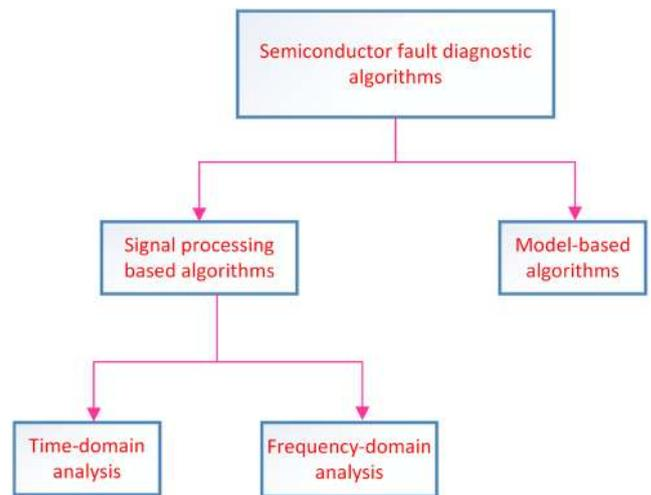
Fig. 2 Categorisation of fault diagnostic algorithms for semiconductor switches in DC–DC converters
