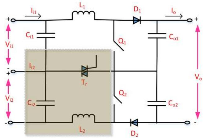
**Fig. 17** Three-level boost converter fault-tolerant structure [44] (grey emphasise box includes new components establish in three-level boost converter)
