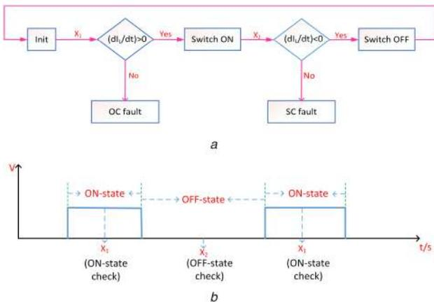
**Fig. 5** Flowchart and gating signals [43]
