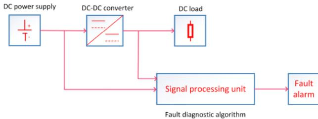
**Fig. 3** Implementation of fault diagnostic algorithm based on signal processing techniques
