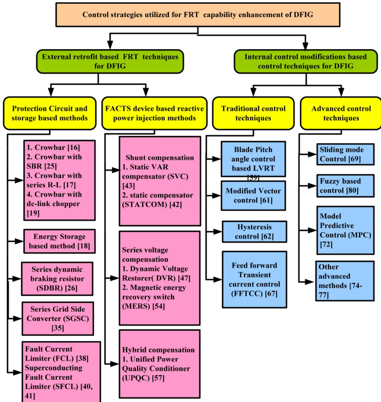
Fig. 3 Classification of FRT capability enhancement techniques for DFIG
