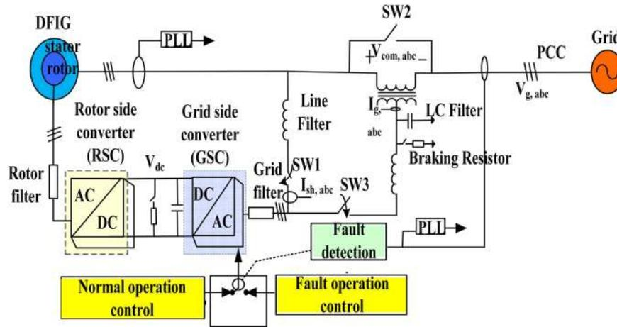
Fig. 10 Schematic representation of DFIG with shunt SGSC
