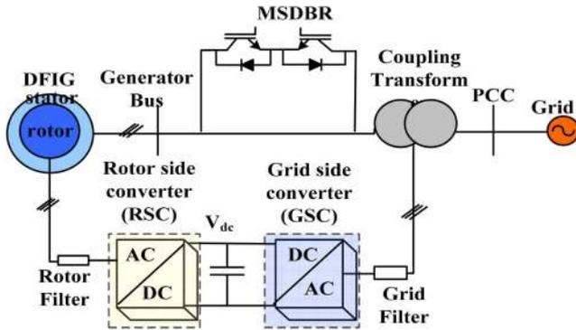
Fig. 8 DFIG-WT equipped with MSDBR
