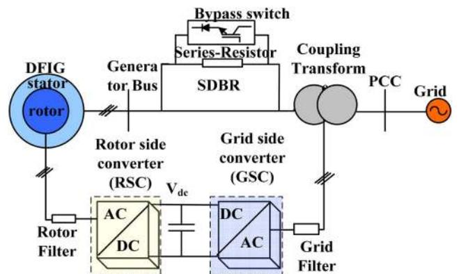
**Fig. 7** DFIG-WT equipped with SDBR
