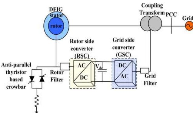
**Fig. 5** FRT capability using crowbar-based methods. Scheme 2 – anti-parallel thyristor-based crowbar
