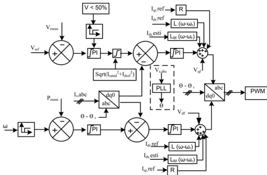
Fig. 19 Configuration of an RSC control configuration in DFIG wind generator
