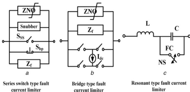
Fig. 12 Generic topologies of SSFCL topologies
