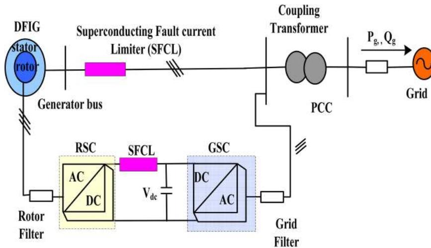
Fig. 11 DFIG with FRT capability using modified flux coupling-type SFCL
