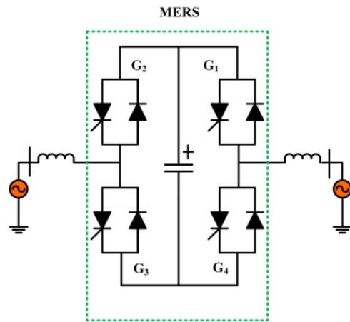
**Fig. 16** Configuration of an MERS as a series FACTS controller device
