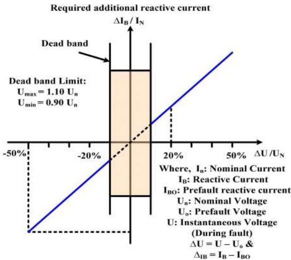
Fig. 2 Reactive power requirement as per E.ON grid code
