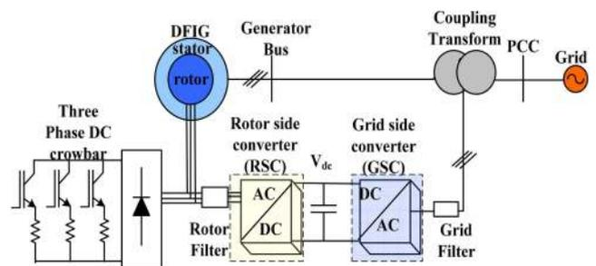
**Fig. 6** FRT capability using crowbar-based methods. Scheme 3 – three-phase DC crowbar
