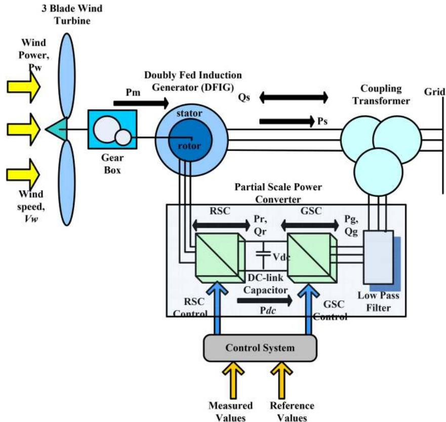
**Fig. 20** Configuration of an RSC and GSC control configuration in DFIG wind generator
