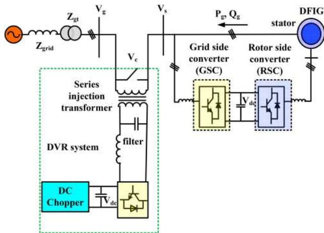
Fig. 15 DVR connected to DFIG
