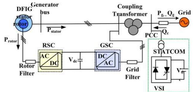
Fig. 13 Placement of STATCOM with DFIG-WT
