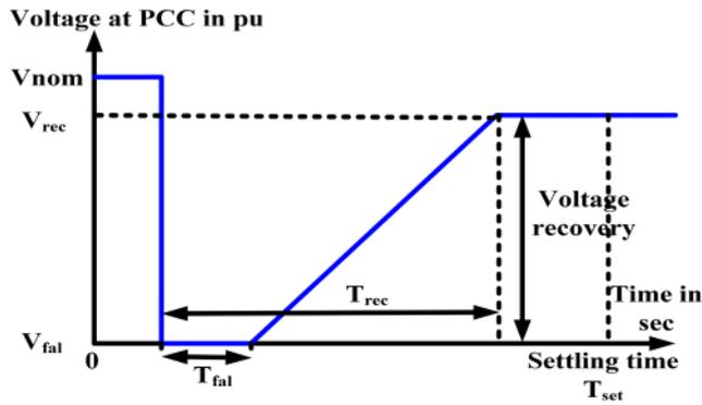
Fig. 1 General FRT capability curve
