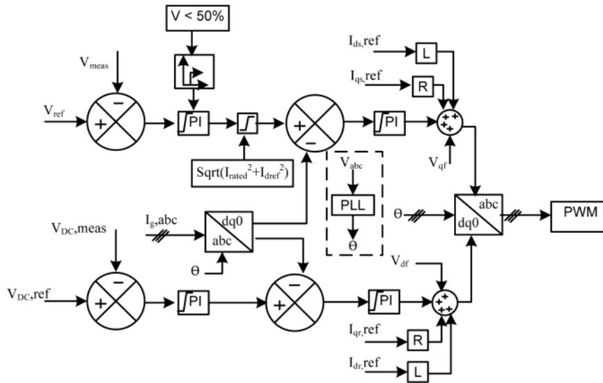
Fig. 18 Configuration of a GSC control configuration in DFIG wind generator
