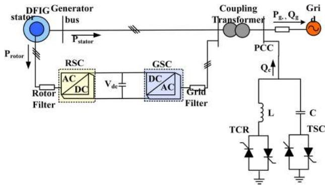
Fig. 14 Placement of SVC with DFIG-WT
