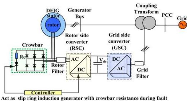
**Fig. 4** FRT capability using crowbar-based methods. Scheme 1 – diode bridge crowbar
