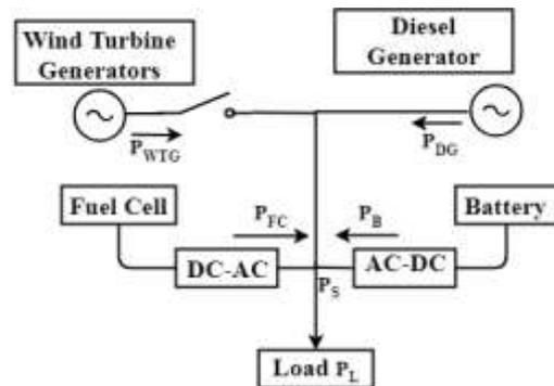
Fig. 1. Schematic diagram of the Hybrid  $\mu G$  System.
