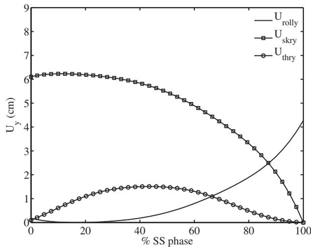
**Fig. 5.** Contributions of each of the segments of the stance leg, i.e., - the rolling foot, shank and thigh to the vertical CoM position. All contributions are scaled such that the lowest value is zero.
