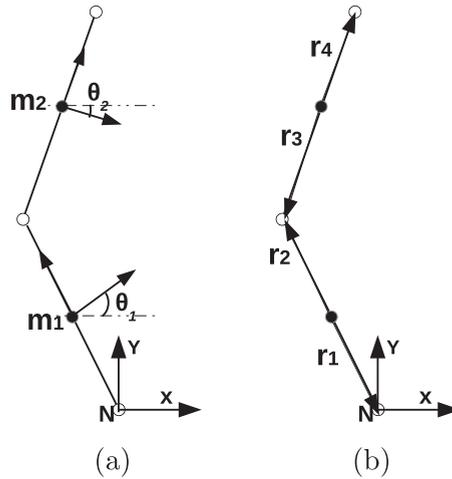
**Fig. B1.** A two-link kinematic chain. (a) shows the body fixed coordinate systems and (segment angles) angles made by the links with respect to the ground and (b) shows the position vectors in local coordinate systems.
