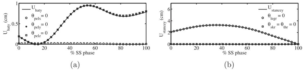
**Fig. 6.** Segmental contribution of the (a) HAT segment to the vertical CoM movement when each of the three DoFs are set equal to zero and that of the (b) segments of the stance leg to the vertical CoM movement when each of the DoFs are set equal to zero. All contributions are scaled such that the lowest value is equal to zero.
