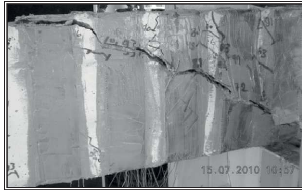
Fig. 6.: Shear failure of Beam 2-1 at load 373.70kN (shear force 122.39kN)
