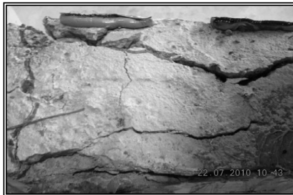
Fig. 9. Crushing of concrete (top-side view) of Beam 2-2
