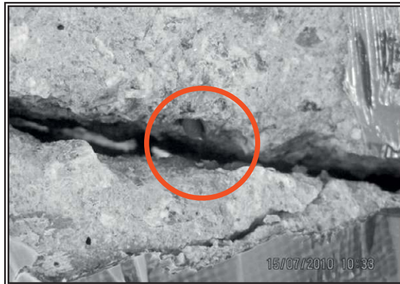
Fig. 6.: Shear failure of Beam 2-1 at load 373.70kN (shear force 122.39kN)
