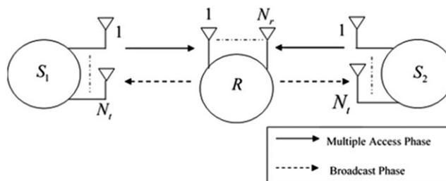
**FIGURE 1** System model for spatial modulation and physical layer network coding-based bidirectional half-duplex relay network with transmit antenna selection
