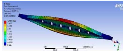
Figure 25. Mode shape 2 of 0.3h 0.5m.
