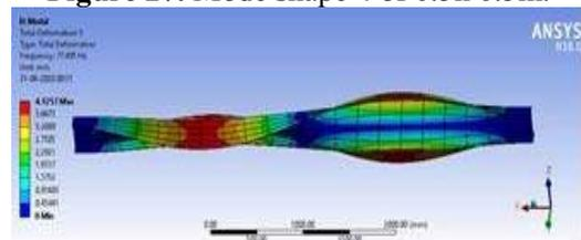
Figure 29. Mode shape 4 of solid beam.
