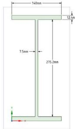
**Figure 3.** Typical beam section details.
