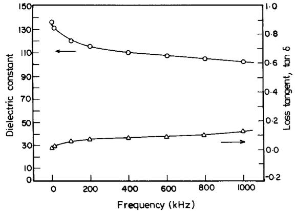
Fig. 4. Variation of dielectric constant and dissipation factor of BTO thin films with frequency.
