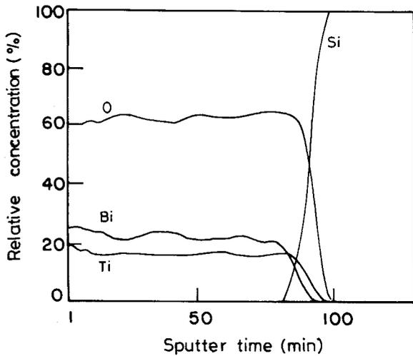
Fig. 3. AES depth profiles of the elements of BTO films annealed at 600°C.
