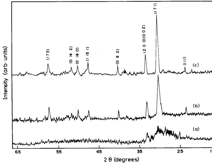
Fig. 1. Powder XRD patterns of BTO thin films annealed at different temperatures for 1 h: (a) 350°C (b) 450°C and (c) 600°C.
