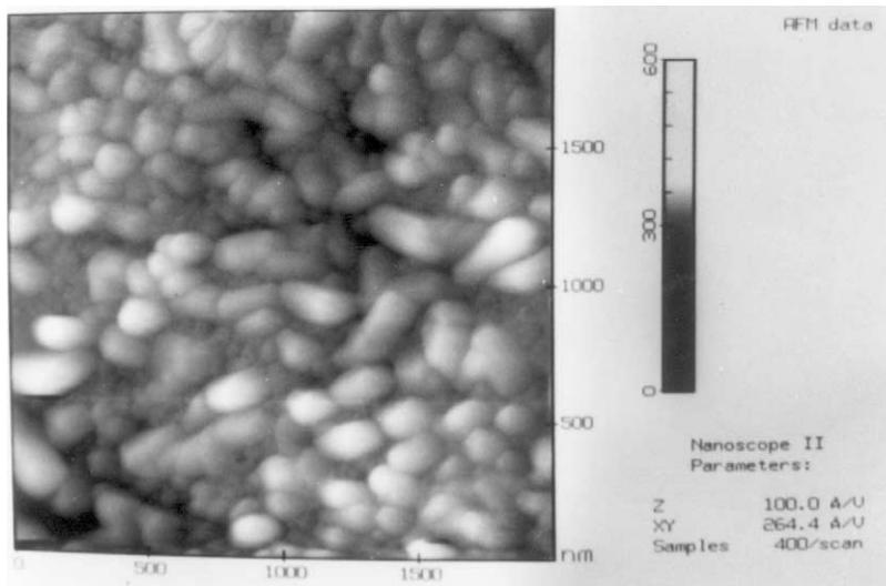
Fig. 2. AFM micrograph of BTO thin film showing uniform grain distribution.
