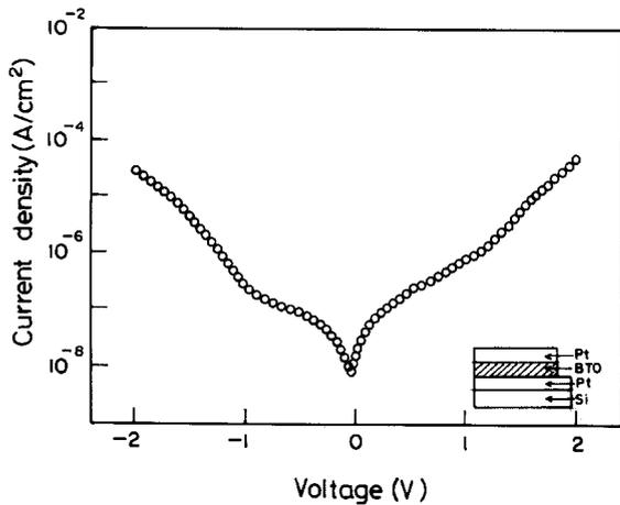
Fig. 6. Leakage current density characteristics of a BTO thin film. The inset shows the M–I–M configuration of the sample used for  $I$ – $V$  measurements.
