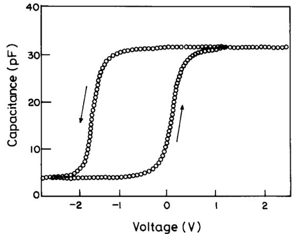
Fig. 5.  $C$ – $V$  characteristics of Pt/BTO/SiO<sub>2</sub>/Si structure with a film thickness of 400 nm.
