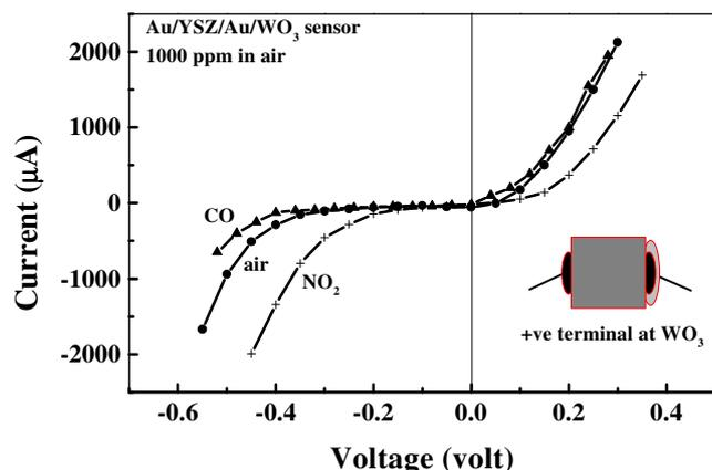
**Figure 4.** Amperometric measurements characteristics of Au/YSZ/Au/WO<sub>3</sub> sensors upon exposure to air and 1000 ppm of NO<sub>2</sub> and CO in air at 650°C.
