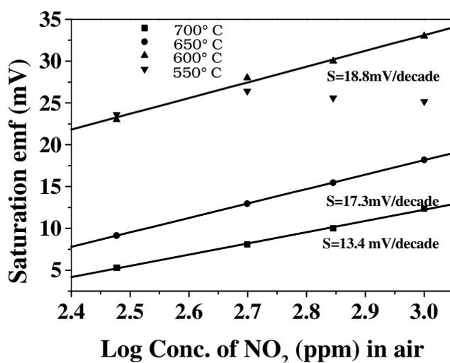
Figure 2. EMF of Pt/YSZ/Pt/WO<sub>3</sub> sensor vs log of NO<sub>2</sub> concentration at different temperatures.
