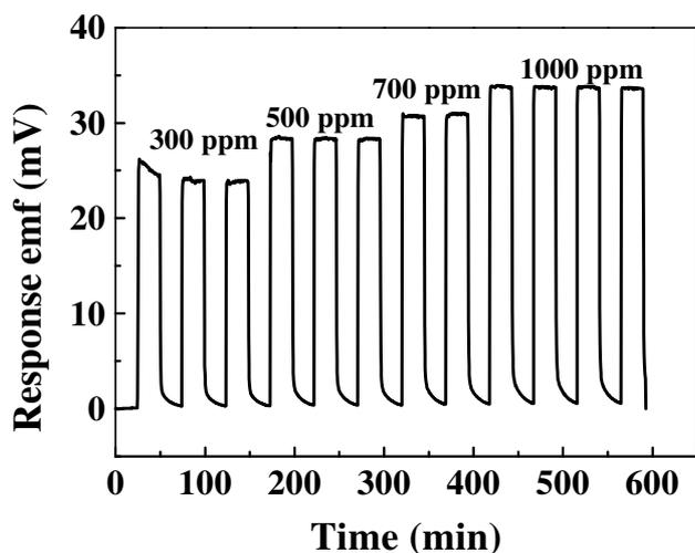
Figure 1. EMF response of Pt/YSZ/Pt/WO<sub>3</sub> sensor at 600°C in cycling air and 100 ppm of NO<sub>2</sub> in air.
