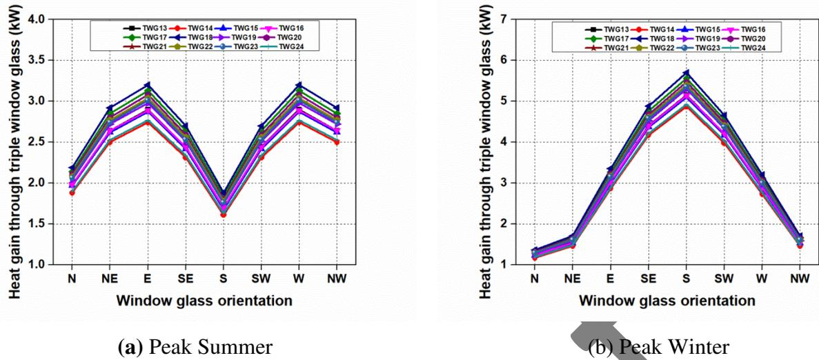
884 **Fig. 6.** Total heat gains (kW) through triple green reflective glass window units in buildings
