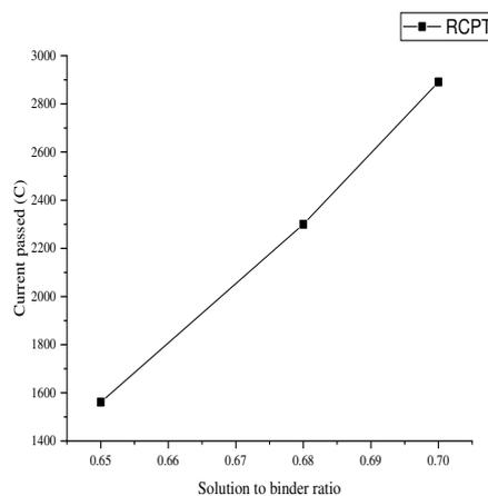
**Figure 2:** Chloride penetration resistance
