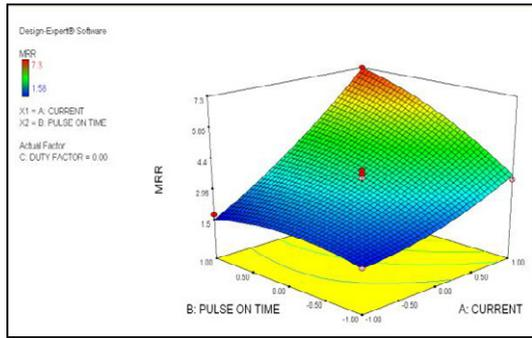
Fig. 6. Surface plot of MRR with current vs. pulse-on-time
