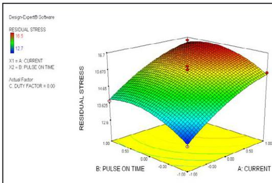
Fig. 8. Surface plot of residual stress vs. current and pulse-on-time
