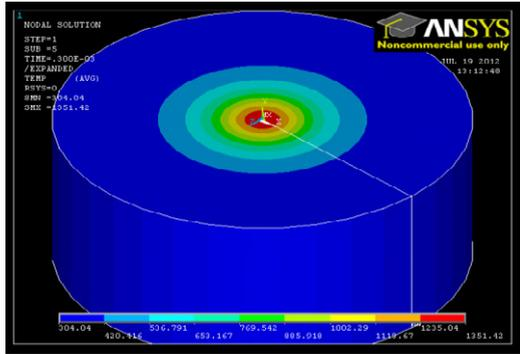
Fig. 4. Temperature distribution on tool at current 7A, spark-on-time 300 μs and voltage 45V
