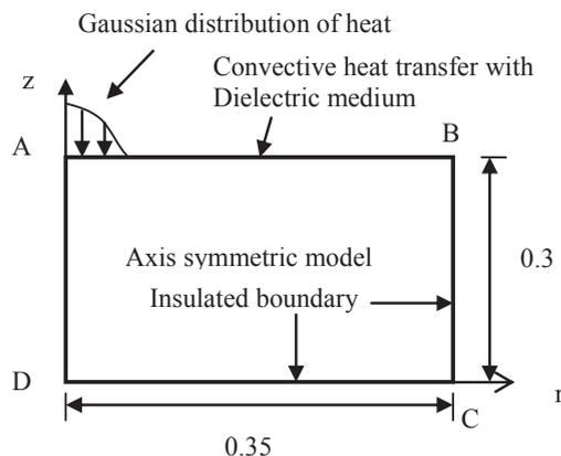
Fig. 1. An axis-symmetric two dimensional model for the EDM process analysis
