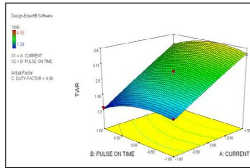
Fig. 7. Surface plot of TWR vs. current and pulse-on-time
