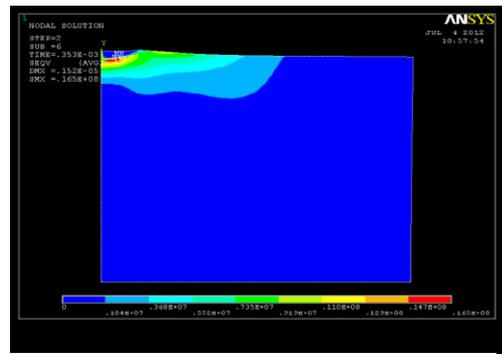
Fig. 5. Residual stress on work piece at current 7A, spark-on-time 300 μs, and voltage 45V
