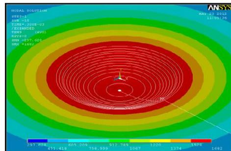
Fig. 3. Predicted crater (depth 13 $\mu$ m, maximum radius 43 $\mu$ m) at current 7A, spark-on-time 300 $\mu$ s, and voltage 45V
