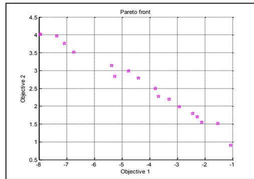
Fig. 9. Pareto-optimal front for objectives MRR and TWR
