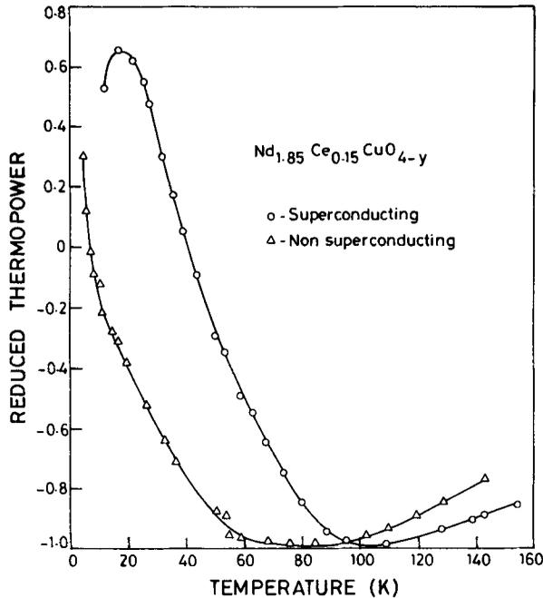
Figure 3. Thermopower vs temperature of  $\text{Nd}_{1.85}\text{Ce}_{0.15}\text{CuO}_{4-y}$ .
