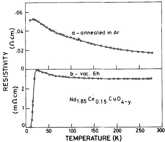
Figure 1. Resistivity vs temperature of  $\text{Nd}_{1.85}\text{Ce}_{0.15}\text{CuO}_{4-y}$ .
