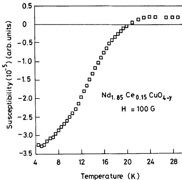
Figure 2. Susceptibility vs temperature of  $\text{Nd}_{1.85}\text{Ce}_{0.15}\text{CuO}_{4-y}$ .
