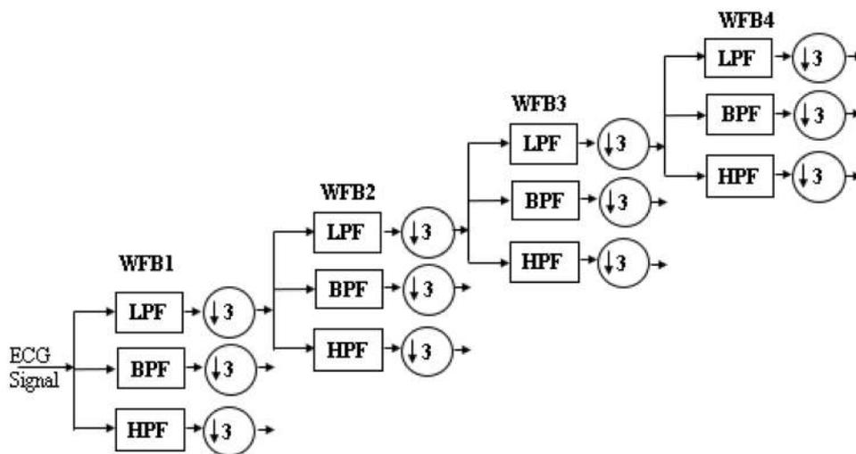
digitized ECG signal into four sub-bands. The transfer function of different filters namely, lowpass, bandpass and highpass, respectively, are obtained as shown in Eqs. (1)–(3).
