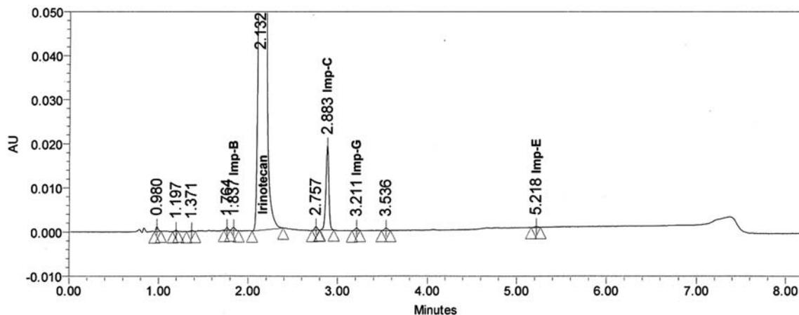
Figure 2. Typical chromatogram of acid degradation sample.
