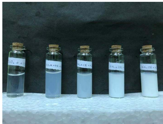
Figure 2: Hybrid Nanofluid Al 2 O 3 /SiO at different concentration
