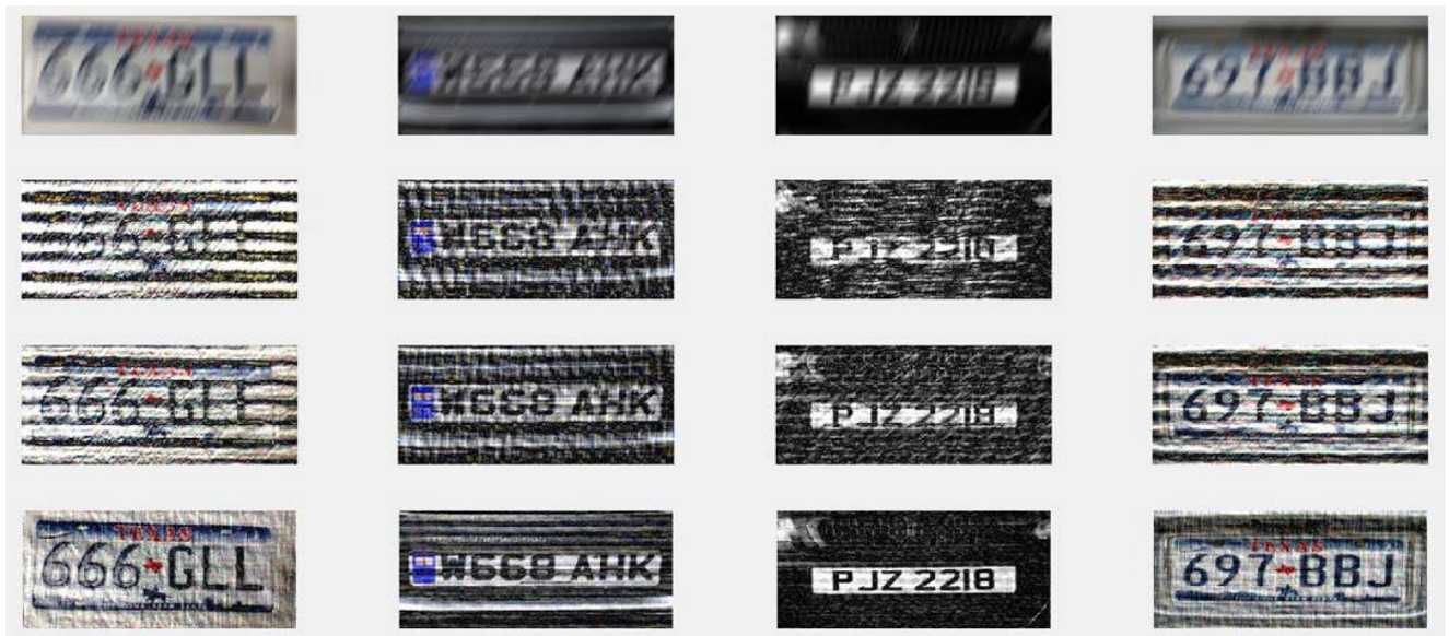
Fig.7. More examples of performances BID schemes: the blurred images are shown in the first row, and the de-blurred results obtained using NSBD [20], RBKE [1] and our method are shown in the second, third and fourth rows respectively.
