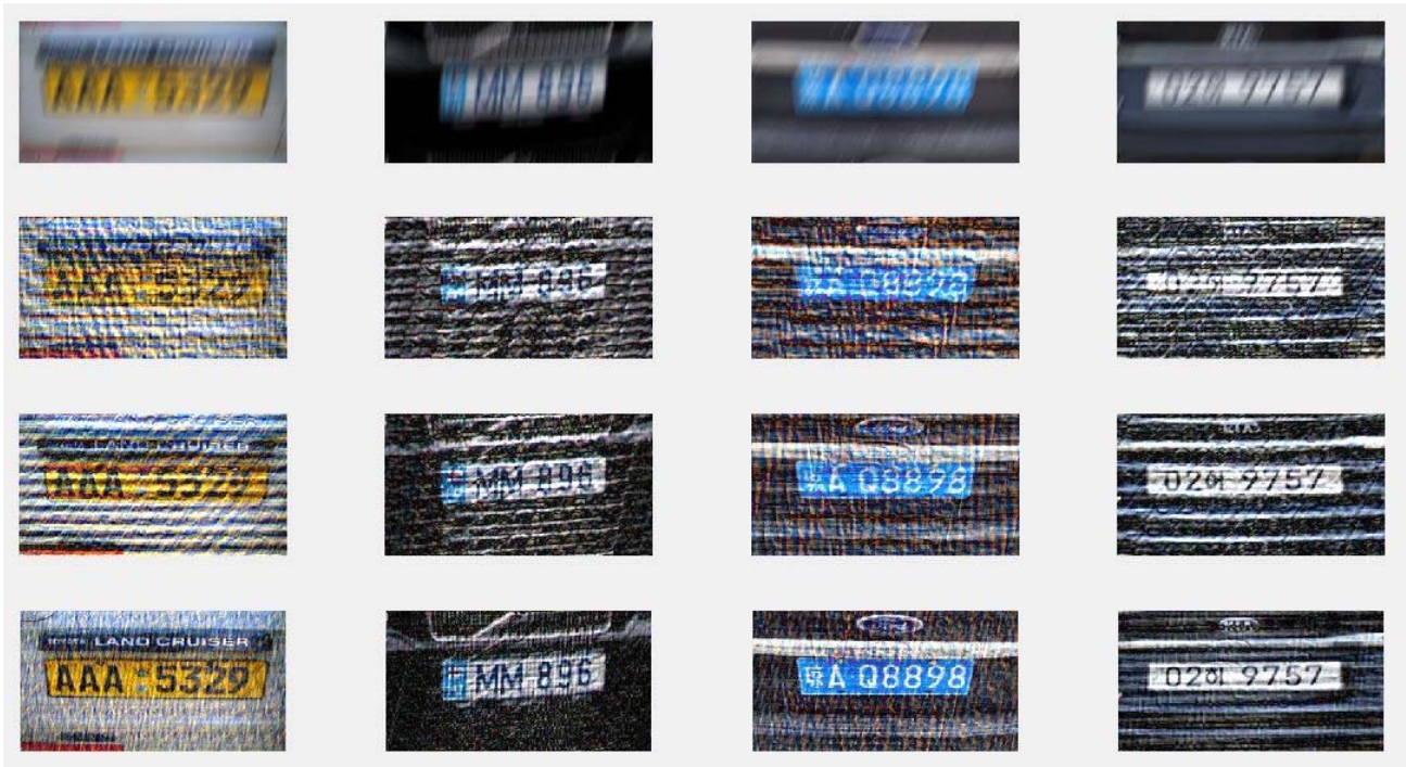
Fig.6. Observed performances of BID schemes: the blurred images are shown in the first row, and the de-blurred results obtained using NSBD [20], RBKE [1] and our method are shown in the second, third and fourth rows respectively.
