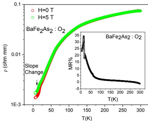
**FIGURE 3.** The results of resistivity vs temperature measurement for  $\text{BaFe}_2\text{As}_2:\text{O}_2$  at  $H = 0$  and 5 T. The inset shows MR as a function of temperature.
