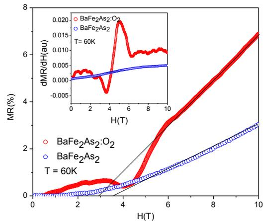
**FIGURE 4.**  $MR$  vs  $H$  for  $\text{BaFe}_2\text{As}_2:\text{O}_2$  and  $\text{BaFe}_2\text{As}_2$ , shown in positive direction, displayed at a representative temperature 60K. The straight line guides the eye for the linear region. The inset shows  $dMR/dH$  vs  $H$  for both.
