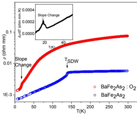
**FIGURE 2.** The results of resistivity vs temperature measurement for  $\text{BaFe}_2\text{As}_2:\text{O}_2$  and  $\text{BaFe}_2\text{As}_2$ . Inset shows  $d\rho/dT$  vs  $T$  for  $\text{BaFe}_2\text{As}_2:\text{O}_2$ .
