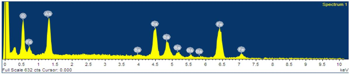
**FIGURE 1.** The results of EDX measurements of  $\text{BaFe}_2\text{As}_2$  single crystals which were kept in air ambience for several months.
