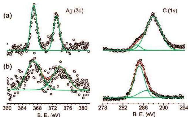
**Figure 2.** Ag(3d) and C(1s) core level spectra of the blend before (a) and after (b) e-beam exposure. The relatively higher spread in data points in (b) is due to poor signal strength as e-beam exposed region was limited to  $3 \times 3 \mu\text{m}^2$ .
