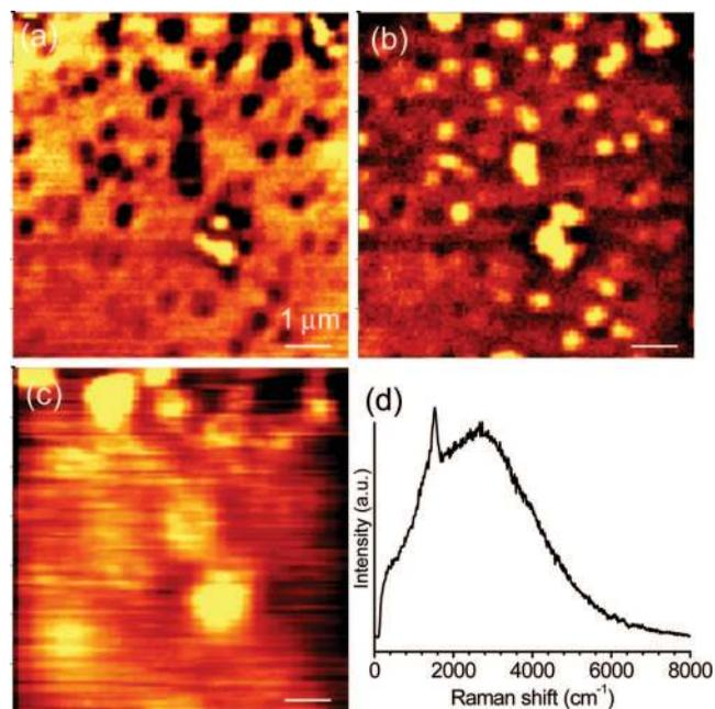
**Figure 6.** (a) Confocal image of Ag nanoparticles in cross-linked polystyrene matrix. Fluorescence (b) and Raman (c) images from the same region. (d) Raman spectrum from the same region. Raman image was acquired using the  $1524\text{ cm}^{-1}$  feature. The images correspond to the same area.
