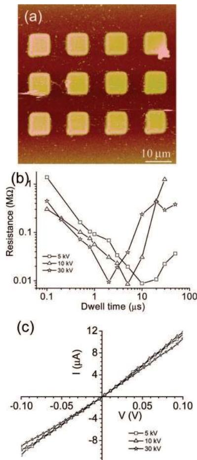
**Figure 7.** (a) AFM image of an array of square islands of the Ag nanoparticles polystyrene composite. (b) Plot of resistance versus dwell time for different islands patterned at 5, 10, and 30 kV. (c)  $I$ - $V$  measurement made using C-AFM showing the lowest resistance obtained with different kVs.
