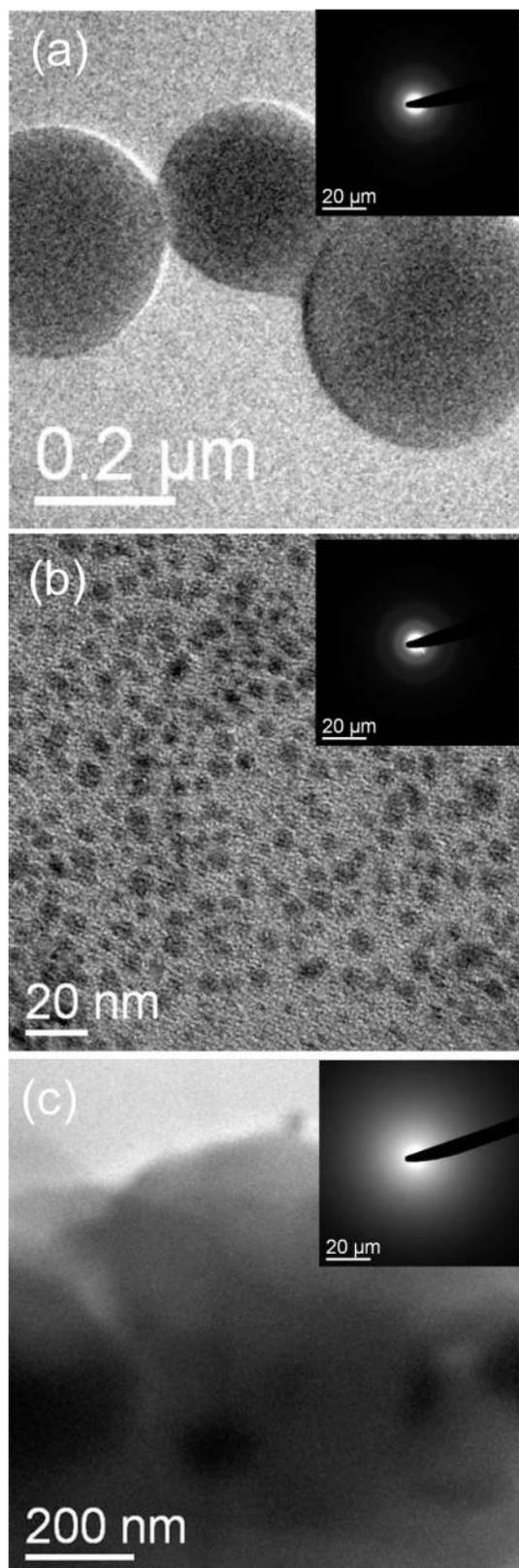
**Figure 9.** TEM images with corresponding ED patterns shown in the inset for patterned regions at 30 kV with different dwell times (a) 0.5, (b) 1, and 50  $\mu\text{s}$ .
