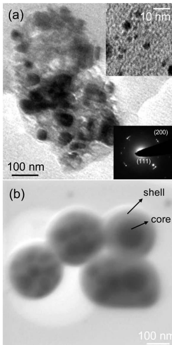
**Figure 4.** (a) TEM image of the e-beam exposed cross-linked blend showing formation of Ag nanoparticles. Inset showing high-resolution image (top) and corresponding electron diffraction pattern (bottom). (b) STEM image of the Ag nanoparticle aggregate. The core and shell regions are marked.
