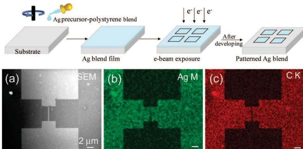
**Figure 1.** Schematic showing the procedure adopted for patterning Ag precursor-polystyrene blend using EBL. Step 1: Spin coating of  $\text{Ag}(\text{PPh}_3)_3\text{NO}_3$ -polystyrene blend on a Si substrate. Step 2: EBL patterning and Step 3: Developing the patterned substrate in *p*-xylene and 2-propanol for 90 and 30 s, respectively. (a) SEM image of a patterned gap electrode. EDS maps obtained using (b) Ag M and (c) C K lines.
