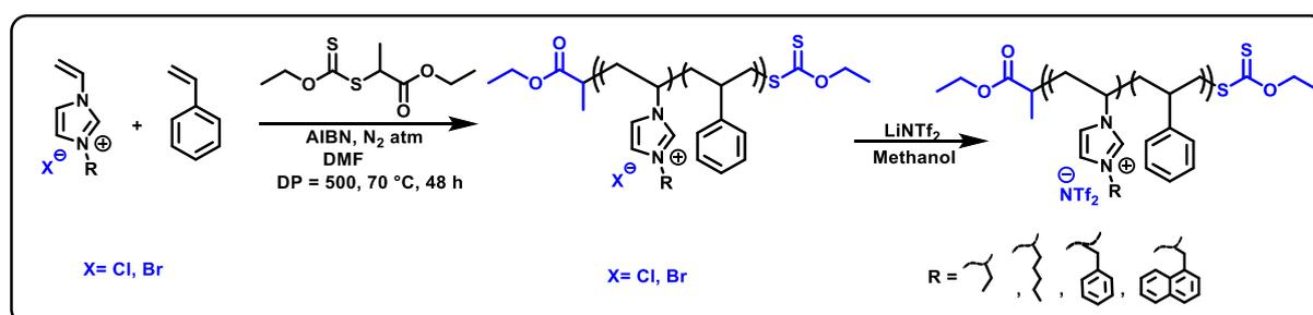
**Scheme 4.** Synthesis of the co-poly(ionic liquid)s [ViRIm](Sty)X.
