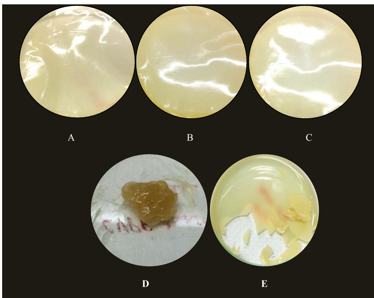
**Figure 2** Pictures of the PIL–IL membranes: (A) poly(ViPenIm)(Sty)NTf<sub>2</sub> with 10 wt% IL, (B) poly(ViBenIm)(Sty)NTf<sub>2</sub> with 25 wt% IL, (C) poly(ViPenIm)(Sty)NTf<sub>2</sub> with 30 wt% IL (D) poly(ViBenIm) NTf<sub>2</sub> with 20 wt% IL (E) poly(ViNapIm) NTf<sub>2</sub> with 20 wt% IL.
