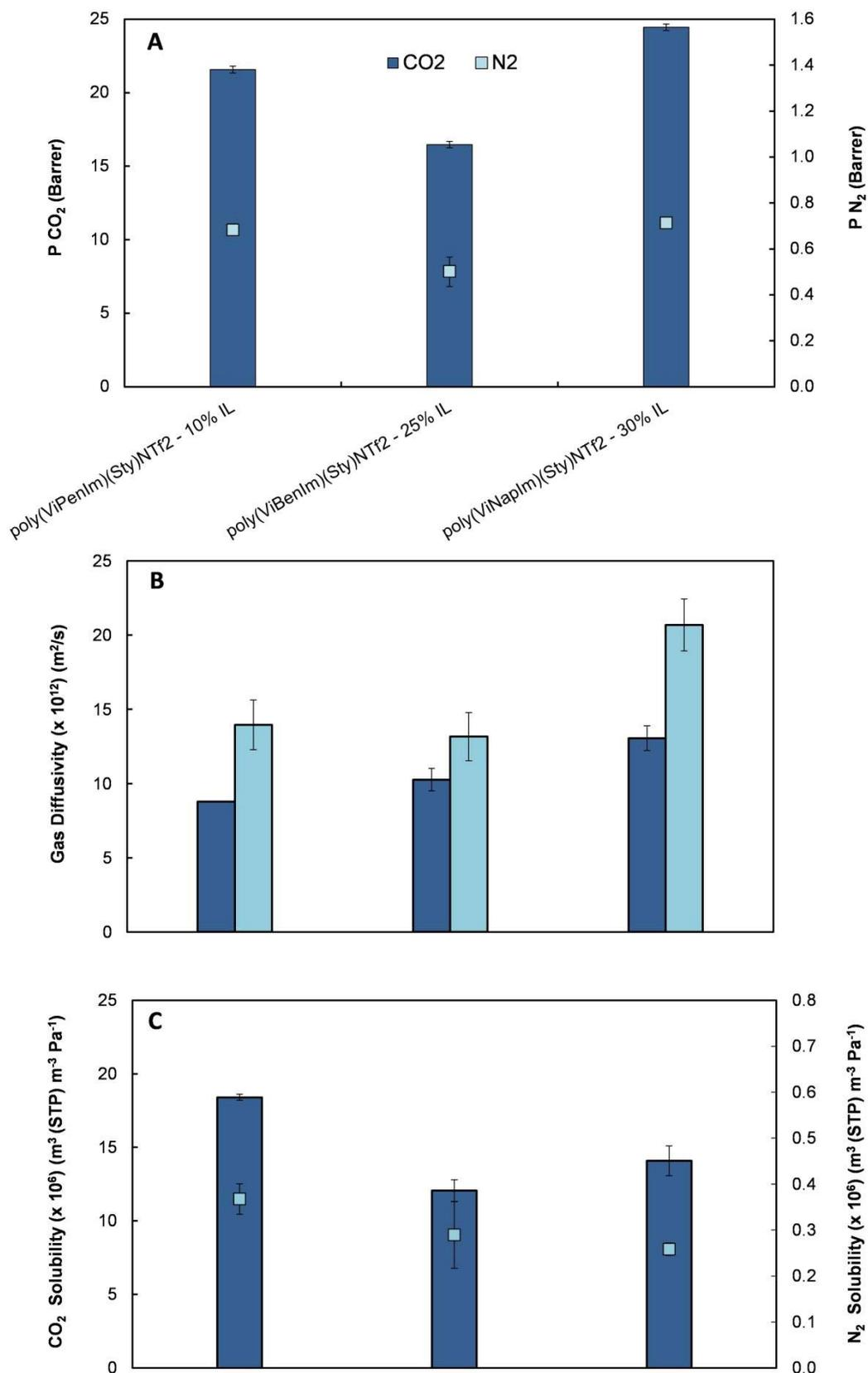
**Figure 3** Gas permeabilities (A), diffusivities (B) and solubilities (C) through the prepared imidazolium-based co-PIL-IL membranes. Error bars represent standard deviations based on three experimental replicas.
