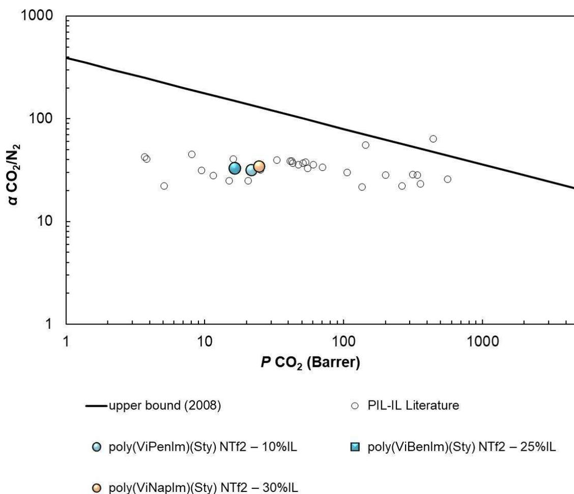
**Figure 4** CO<sub>2</sub>/N<sub>2</sub> separation performance of the co-PIL–IL composite membranes obtained in this work. Data is plotted on a log-log scale and the upper bound is adapted from Robeson.<sup>53</sup> Literature values of other PIL–IL composite membranes previously reported are also illustrated for comparison.<sup>23, 30, 32, 38, 40, 47, 54</sup>
