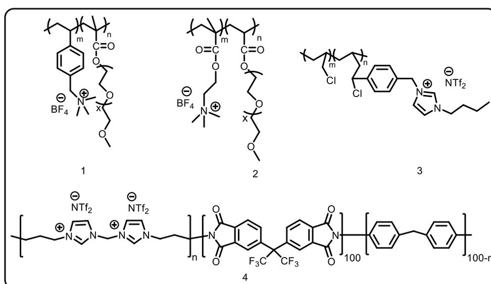
**Figure 1** Different PIL copolymers structures which have been used to develop CO<sub>2</sub> separation membranes.
