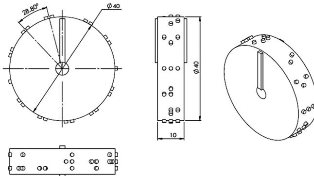
**Fig. 2.** Modified 12 letter embossed disc (dimensions in mm)
