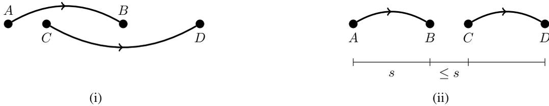
Fig. 1. Conditions under which receiver  $B$  experiences interference due to transmitter  $C$ .
