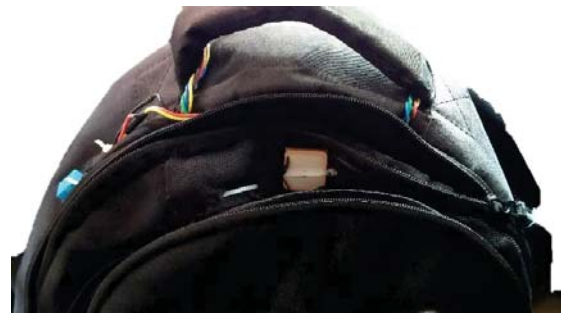
Fig 10. A top view of the bag showing the integration of the DHT11 temperature and humidity sensor and the GPS Module.
