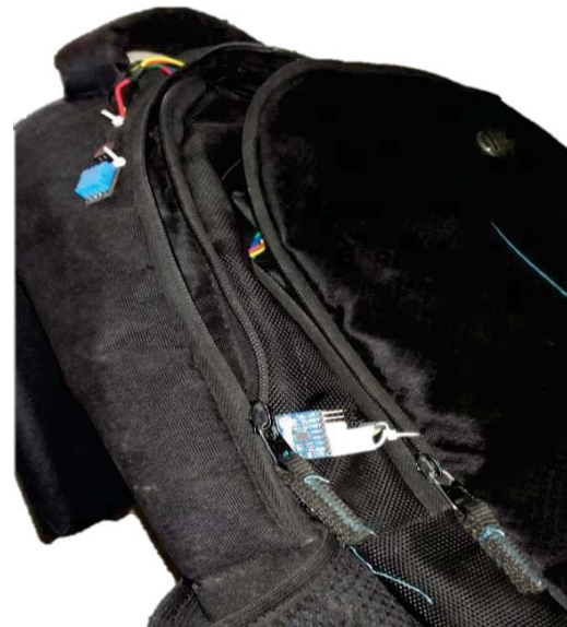
Fig 11. A side view of the bag showing the integration of the DHT11 temperature and MPU6050 IMU Sensor.
