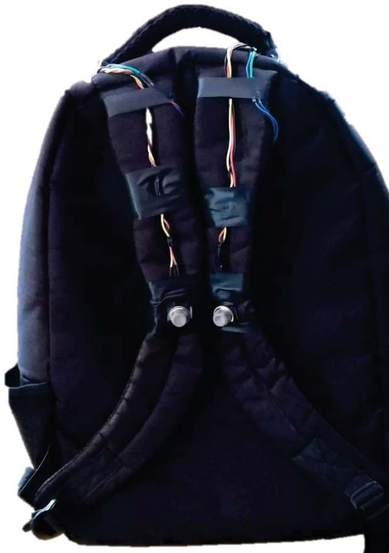
Fig 9. A rear view of the bag which shows the integration of piezo sensors, SOS button, Gas Sensors on the straps of the bag.
