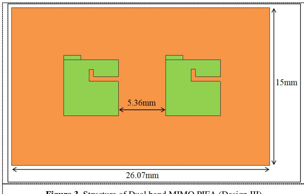
**Figure 3.** Structure of Dual band MIMO PIFA (Design III).
