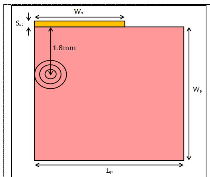
**Figure 1.** Structure of Single band PIFA (Design I).
