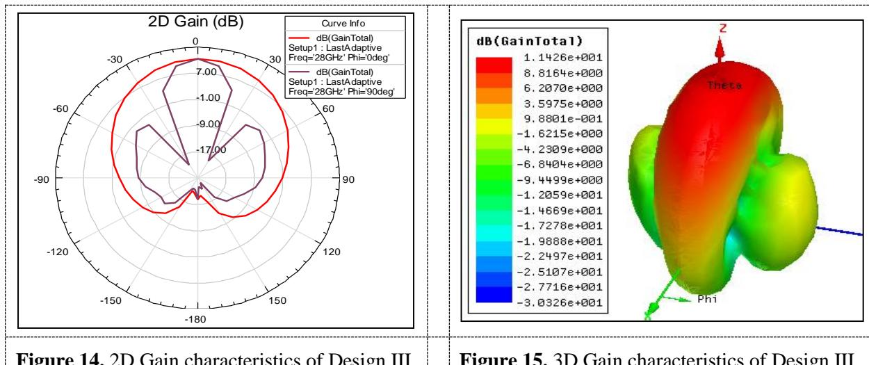
**Figure 14.** 2D Gain characteristics of Design III.**Figure 15.** 3D Gain characteristics of Design III.
