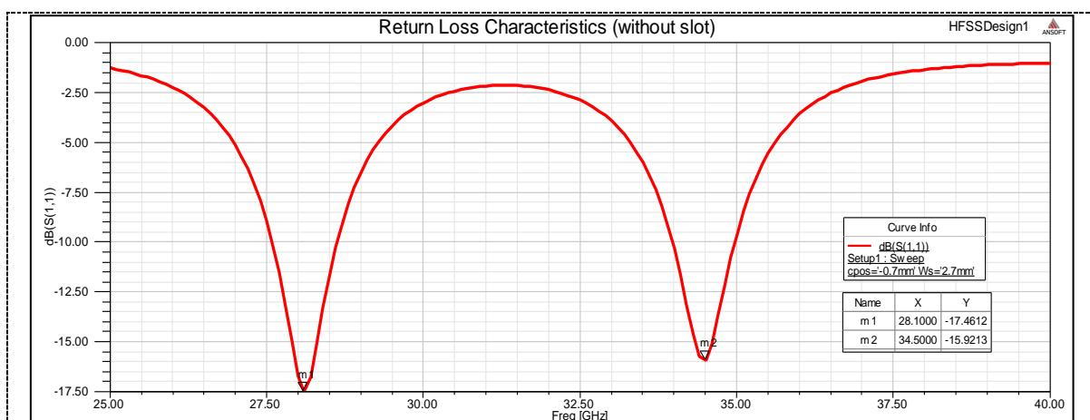
**Figure 5.** Return loss characteristics of Design I.
