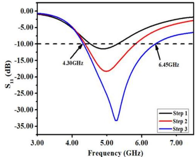
Fig. 2. Comparison of Reflection Coefficients ( $S_{11}$ ) of different steps involved in antenna design.
