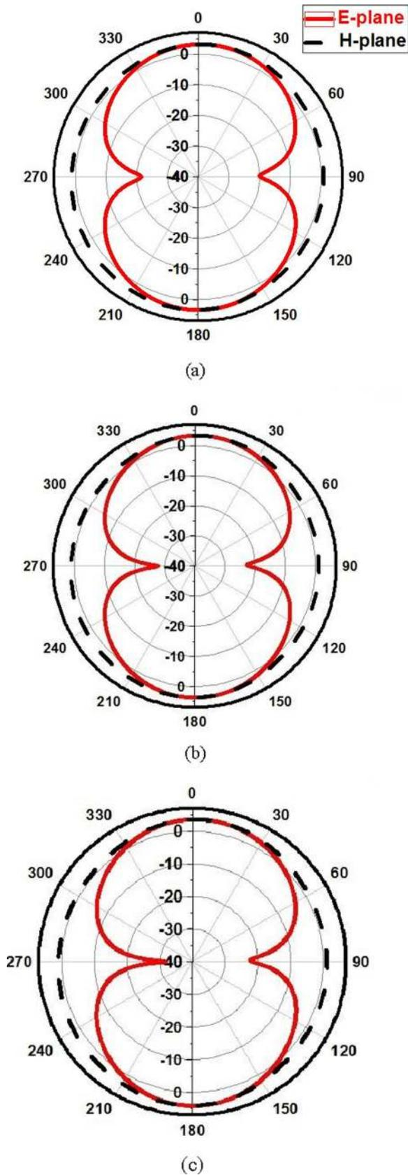
Fig. 12. Simulated radiation pattern of the proposed configuration at (a) 5, (b) 5.2 and (c) 5.8 GHz.
