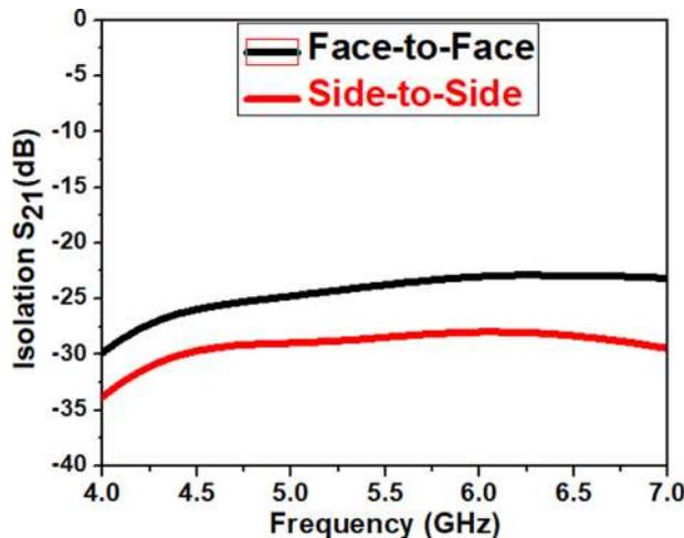
Fig. 17. Isolation analysis of the designed antenna.
