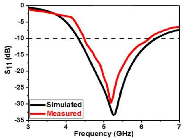
Fig. 8. Simulated and measured S<sub>11</sub> of the final antenna.
