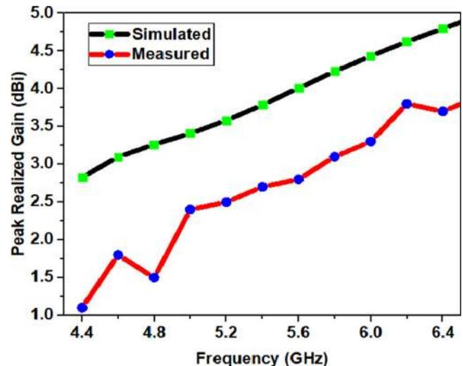
Fig. 11. Simulated and measured peak realized gain of the proposed configuration.
