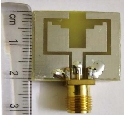
Fig. 4. Fabricated antenna.
