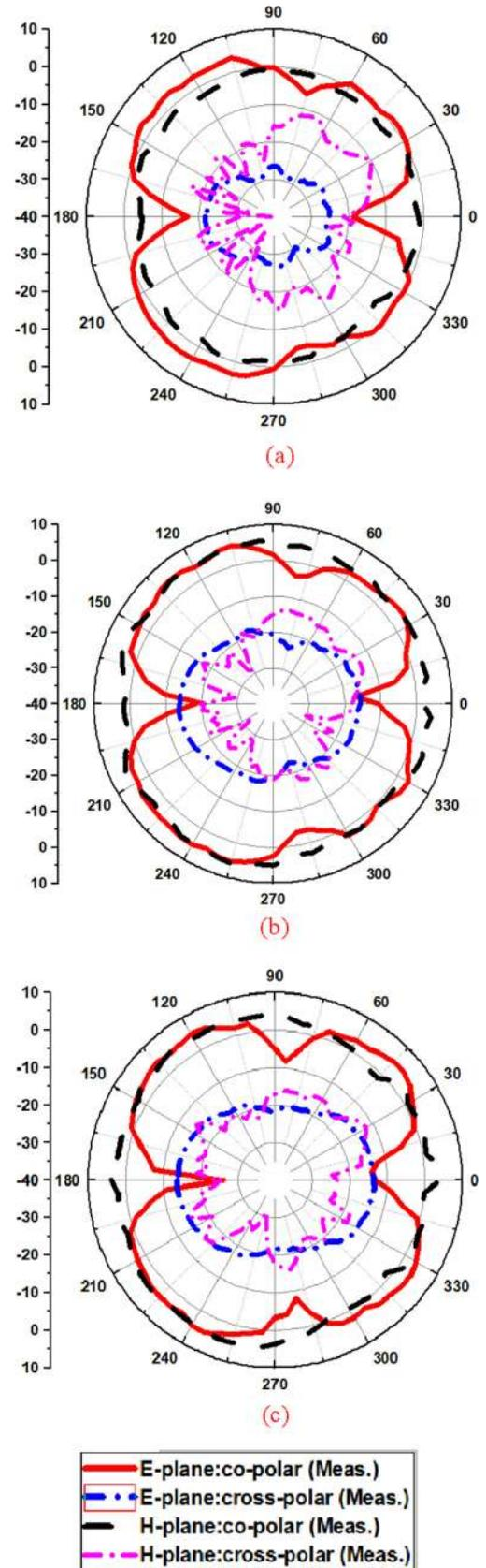
Fig. 13. Measured radiation pattern of the proposed configuration at (a) 5, (b) 5.2 and (c) 5.8 GHz.
