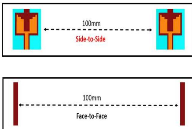
Fig. 14. Side-to-side and Face-to-Face orientations of antenna setup in HFSS to measure time domain characteristics.
