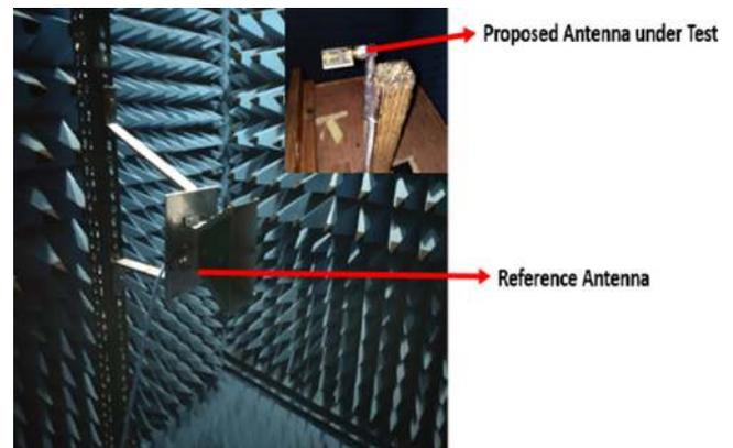
Fig. 10. Gain and radiation pattern measurement set up in anechoic chamber.
