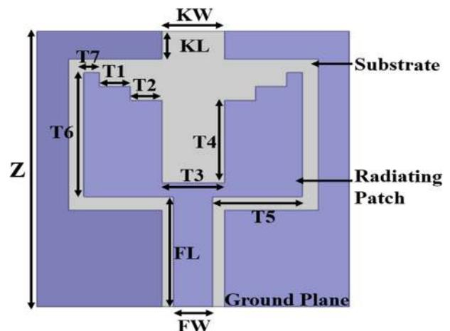
Fig. 3. Proposed antenna structure front plane.
