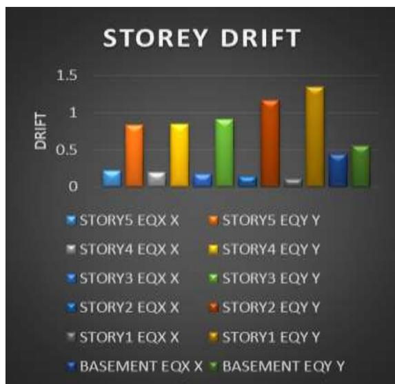
Fig 9: Storey drift of 275 mm thick RCC shear wall
