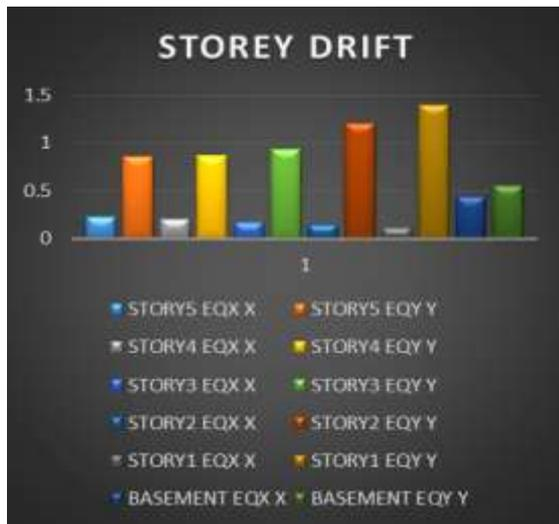
Fig 8: Storey drift of 250 mm thick RCC shear wall
