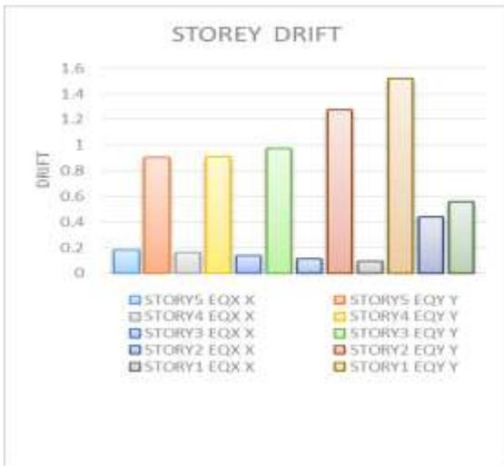
Fig 16: Storey drift of 24 mm thick composite shear wall
