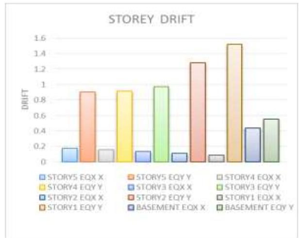
Fig 18: Storey drift of 28 mm thick composite shear wall
