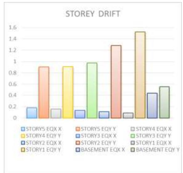
Fig 17: Storey drift of 26 mm thick composite shear wall
