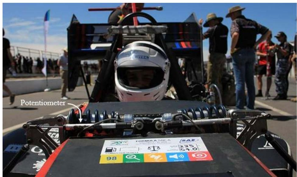
bar sustain an impact. The potentiometer mounted on the vehicle is depicted in Fig. 17.
