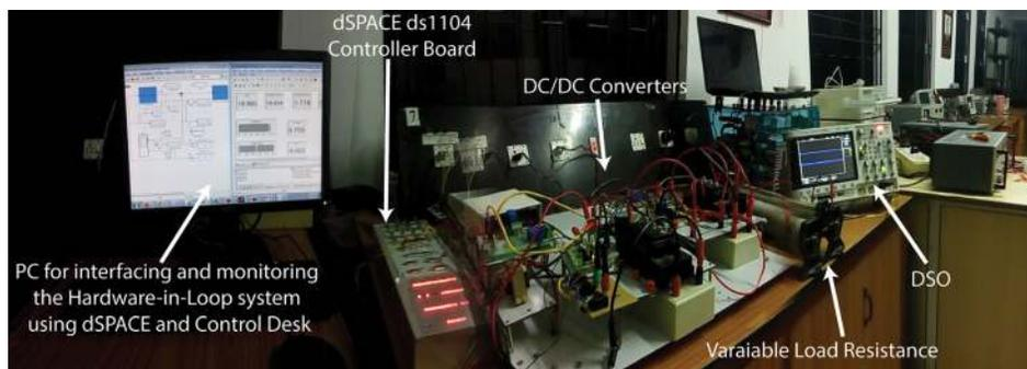
FIG. 10. Hardware setup of solar PV emulator.
