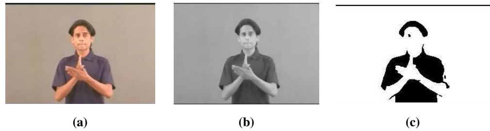
Figure 4. Sign gesture recognition for meat : (a) input frame, (b) noise removed, output, (c) segmented output.
