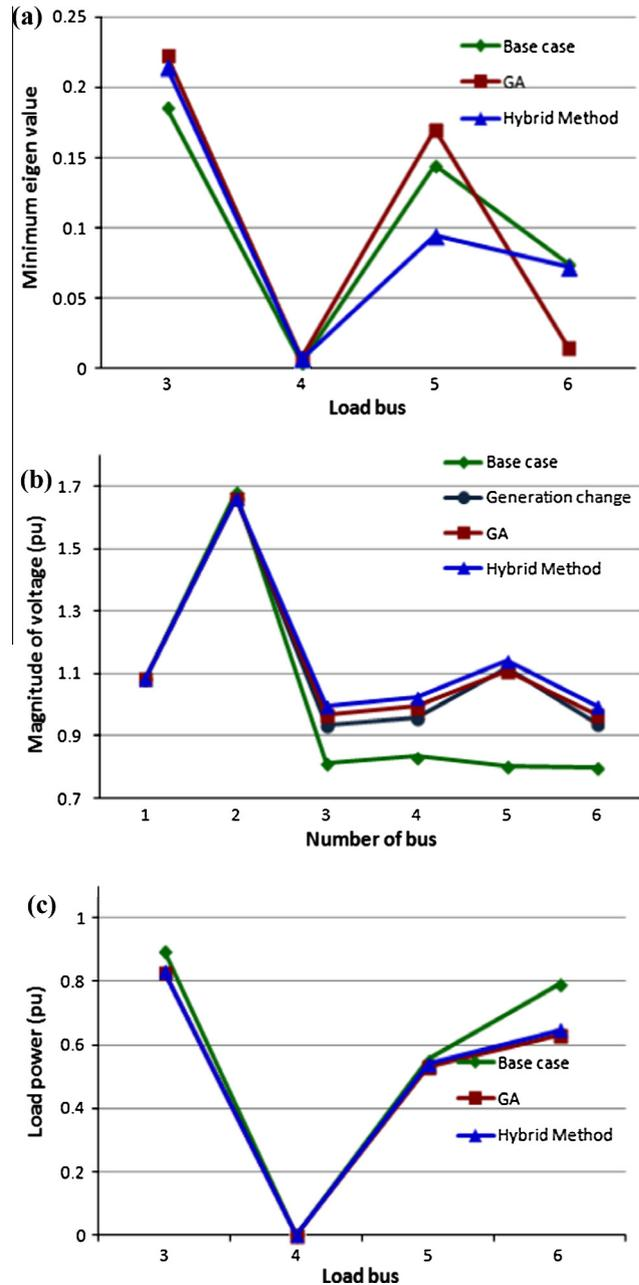
**Figure 4** Six bus system performance comparison: (a) minimum eigenvalue, (b) magnitude of voltage (pu) and (c) load power (pu).
