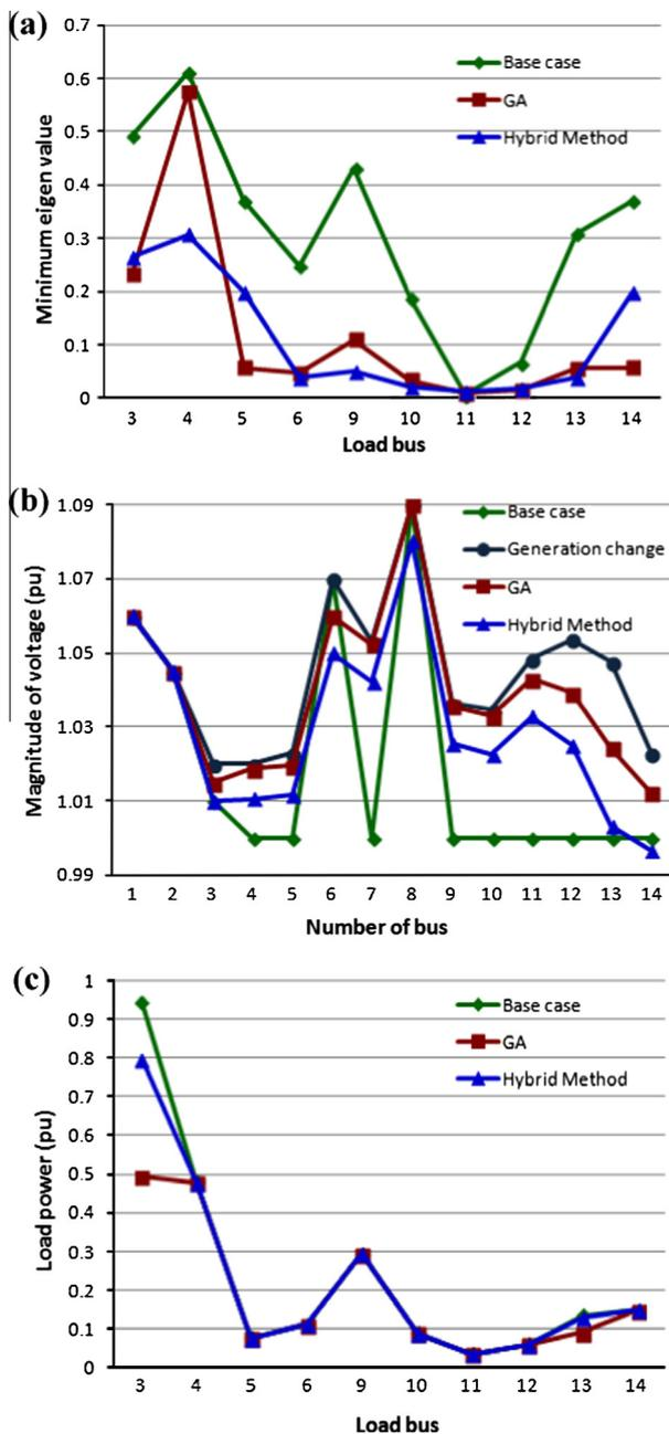
Figure 5 IEEE 14 bus system performance comparison: (a) minimum eigenvalue, (b) magnitude of voltage (pu) and (c) load power (pu).
