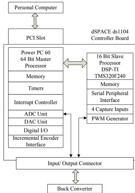
Fig. 3 Block Diagram of ds1104 Processor Board
