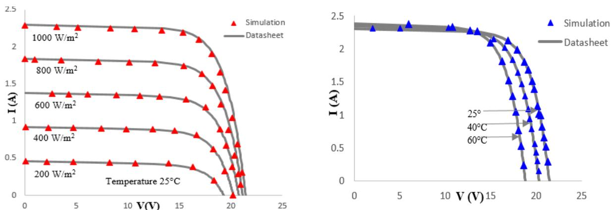
Fig.2. Comparison of simulated I-V curves with datasheet values of Shell S36 Solar PV Panel under different irradiation and temperature
