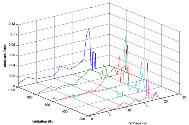
Fig. 7 a. Comparison of Experimental values with datasheet values at different irradiation
