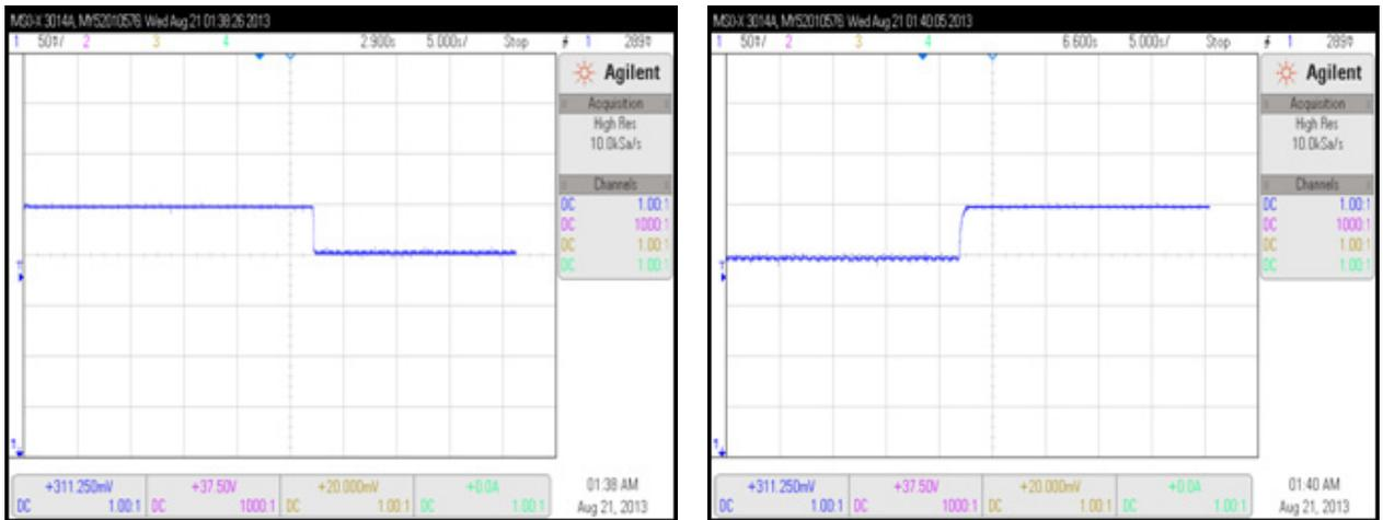
Fig. 8 a. and b. Dynamic response for sudden change in irradiation from 1000 to 200W/m<sup>2</sup> and 200 to 1000 W/m<sup>2</sup> with constant temperature respectively.
