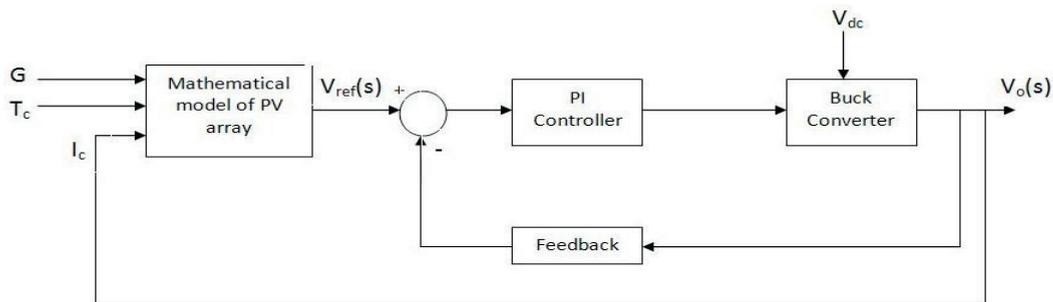
Fig. 5 Feedback Control system of DC-DC Buck converter
