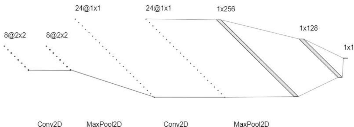
**Figure 2.** The architecture of the CNN that was developed for this application. Although the depth is shown as 8 and 24 it is only indicative. Every layer has a depth of 3005 indicating the number of datapoints in the training dataset.
