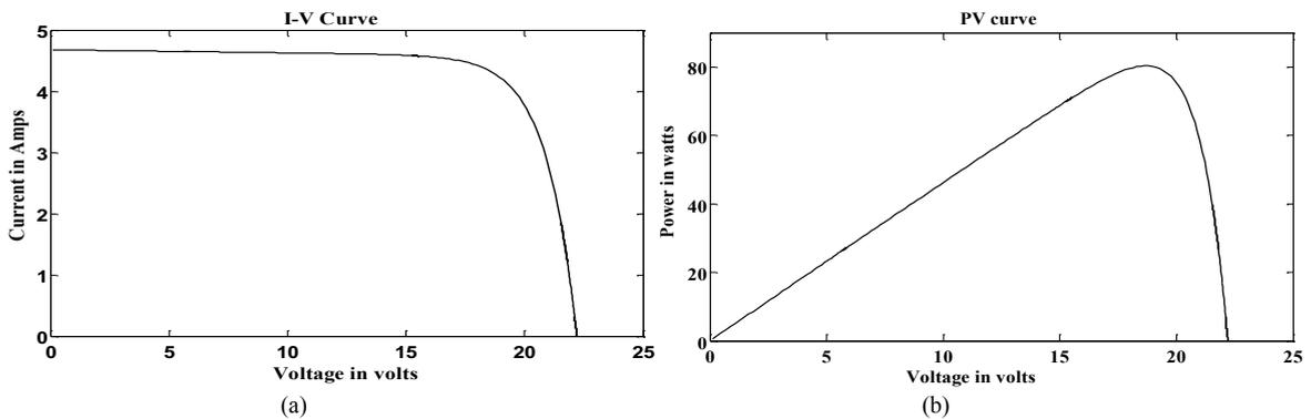
Fig. 3 (a) I-V & (b) P-V characteristics
