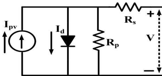
Fig. 2 Single diode model equivalent circuit
