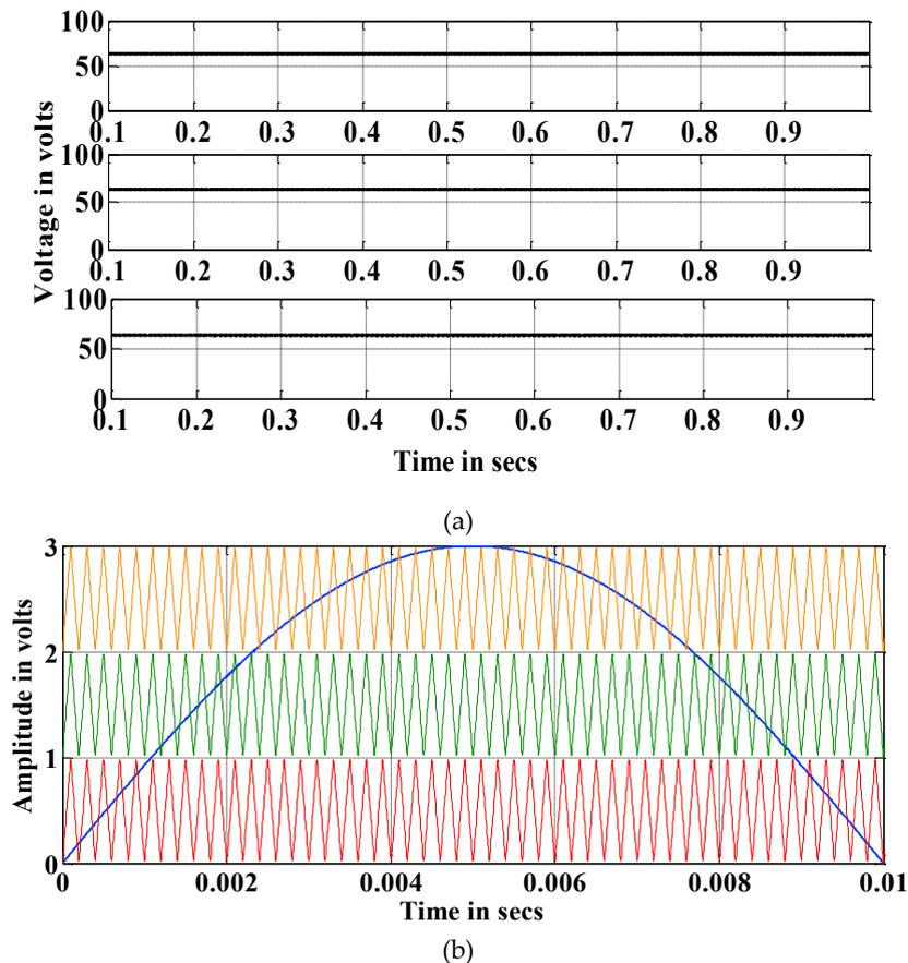
Fig. 5. (a) Multi Output voltage of boost converter (b) Unipolar Phase Disposition PWM
