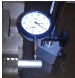
Fig. 16. Runout measurement using a dial indicator.
