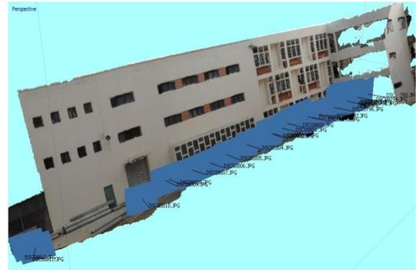
**Figure 5:** Building façade with video frame positions
