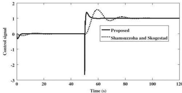
Figure 14: Control signal of example 4 for perturbed response.
