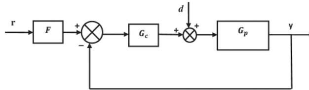
Figure 1: Proposed control structure.
