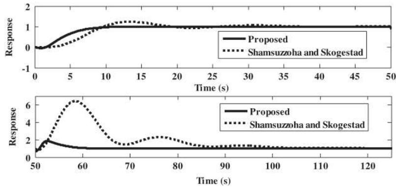
Figure 12: Servo and regulatory responses of example 4 under perturbed conditions.
