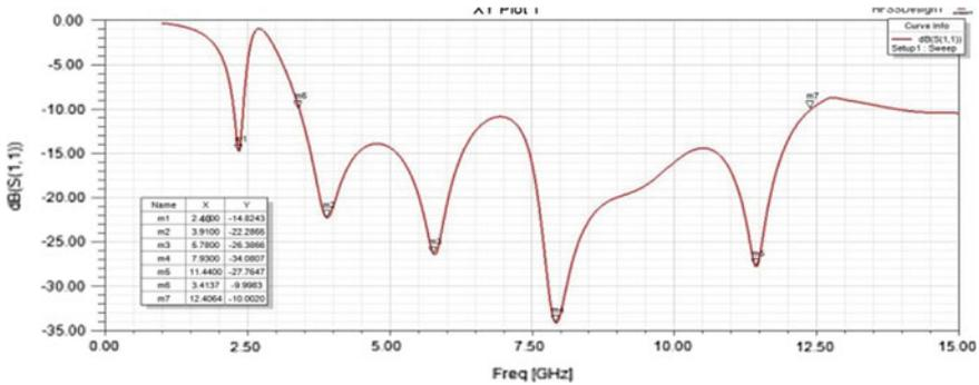
Fig. 8 Return loss of the modified antenna
