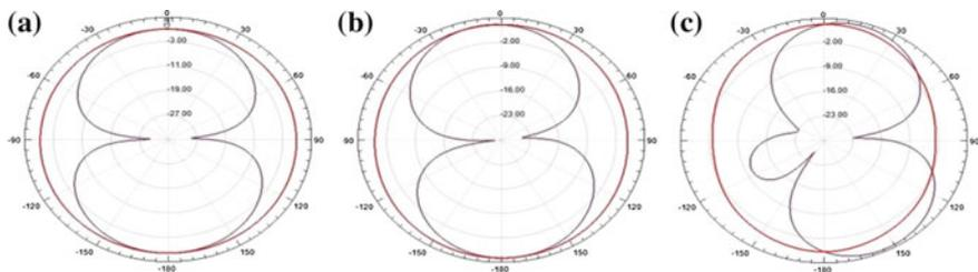
**Fig. 16** Radiation patterns of UWB circular fractal antenna with Tripole-pair FSS at **a** 3.5 GHz, **b** 6 GHz, **c** 9 GHz
