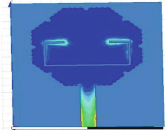
**Fig. 10** Current distribution on the modified antenna
