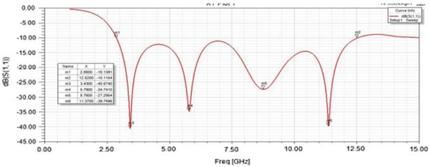
Fig. 3 Return loss of the planar monopole antenna
