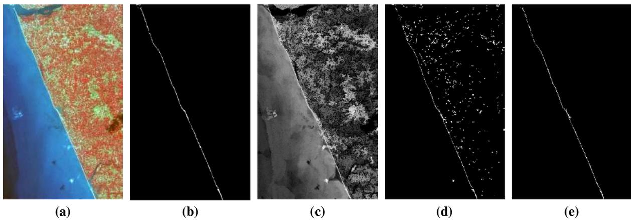
**Figure 4.** Illustration of results with Resource sat-2, LISS IV imagery. (a) Original image, (b) Ground truth, (c) MM processed image (intermediate stage), (d) Classification outcome, (e) Proposed MM algorithm outcome.
