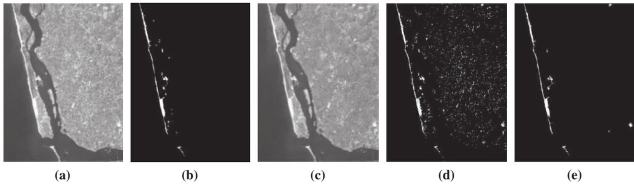
**Figure 3.** Illustration of results with Cartosat-2 imagery (a) Original image, (b) Ground truth, (c) MM processed image (intermediate stage), (d) Classification outcome, (e) Proposed MM algorithm outcome.
