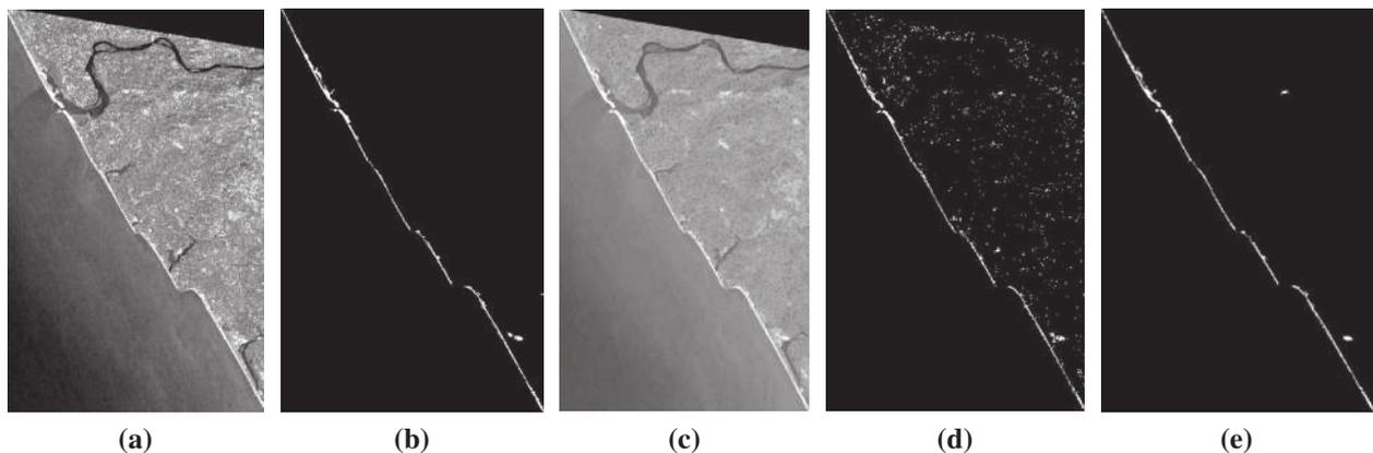
**Figure 2.** Illustration of results with Cartosat-1, PAN (Tile-532-338) imagery. (a) Original image, (b) Ground truth, (c) MM processed image (intermediate stage), (d) Classification outcome, (e) Proposed MM algorithm outcome.
