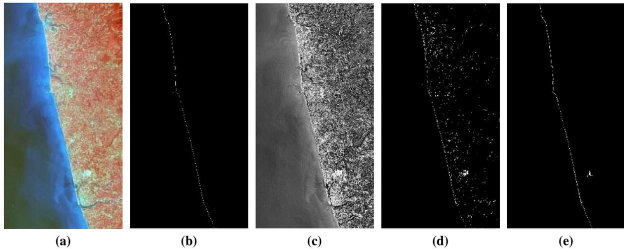
**Figure 6.** Illustration of results with Landsat ETM + sensor imagery. (a) Original image, (b) Ground truth, (c) MM processed image (intermediate stage), (d) Classification outcome, (e) Proposed MM algorithm outcome.
