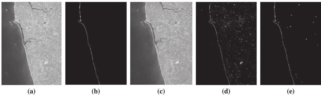
**Figure 5.** Illustration of results with Cartosat 1, PAN (Tile-530-334) imagery. (a) Original image, (b) Ground truth, (c) MM processed image (intermediate stage), (d) Classification outcome, (e) Proposed MM algorithm outcome.
