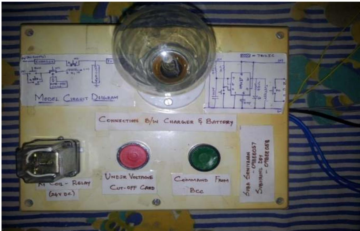
Fig. 4: Prototype for the overall schematics
