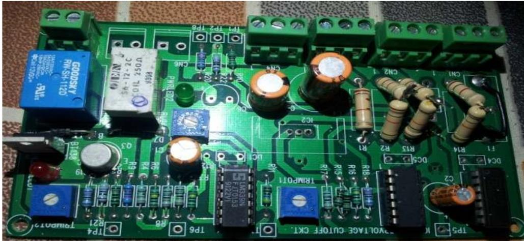
Fig. 8: Under-voltage cut-off card
