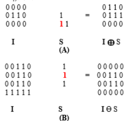
Fig. 1: Dilation and Erosion for Small Image A. Dilation, B. Erosion.
