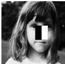
Figure 2. Shows the application of Haar Feature on an image of identifying a nose (From Bing)
