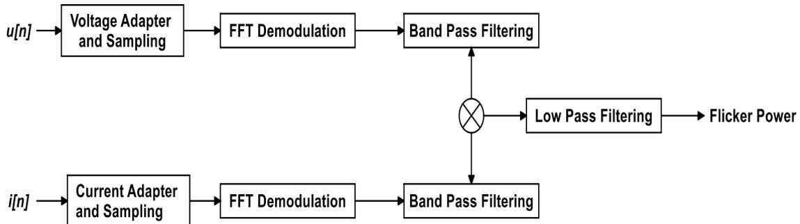
Figure 14. FFT demodulation algorithm for flicker power calculation
