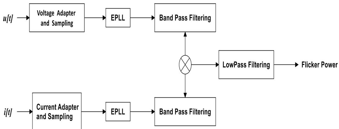
Figure 15. Block diagram of flicker detection by enhanced phase locked loop method
