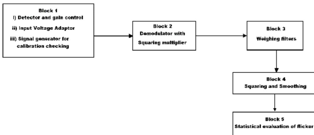
Figure 1. Block diagram of IEC flicker meter
