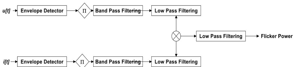
Figure 5. Block diagram to calculate flicker power
