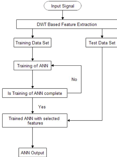
Figure 20. Block diagram of DWT-ANN method for identification
