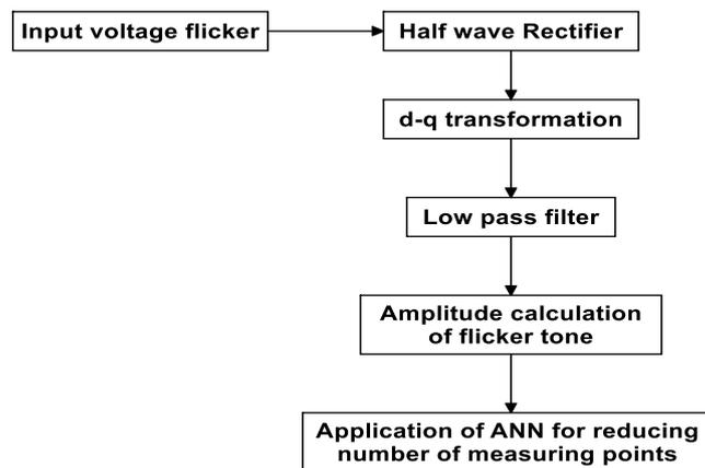
Figure 13. Block diagram of D-Q transformation method for magnitude calculation
