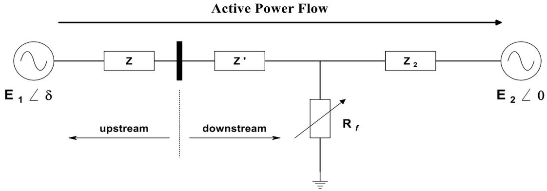
Figure 2. Equivalent Circuit for Analysis of Flicker Source Detection by Slope Method
