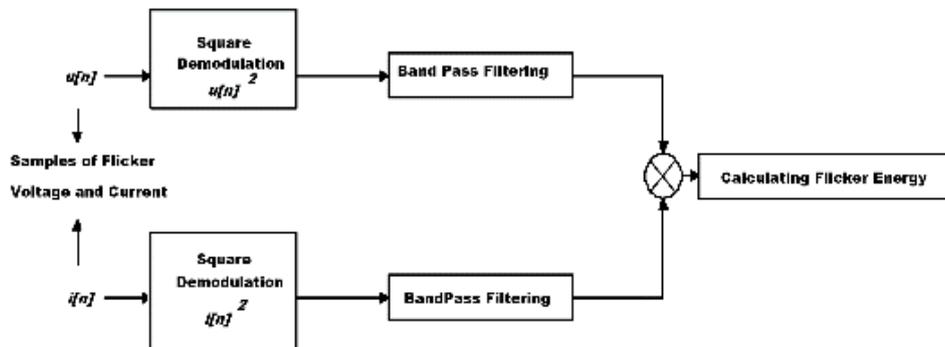
Figure 4. Block diagram for calculation of flicker energy
