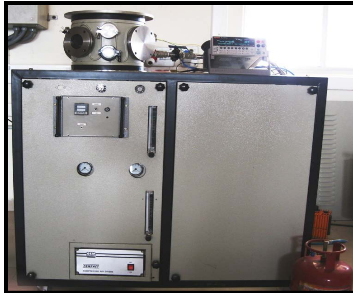
Fig 16 Gas sensor setup used for LPG sensitivity measurement
